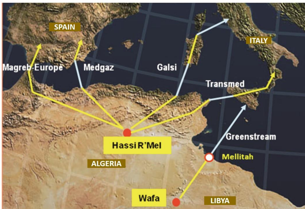
Five submarine pipelines connect the south and the north coasts of the Mediterranean basin delivering the Algerian and Libyan natural gas to Europe (Created by the author)
