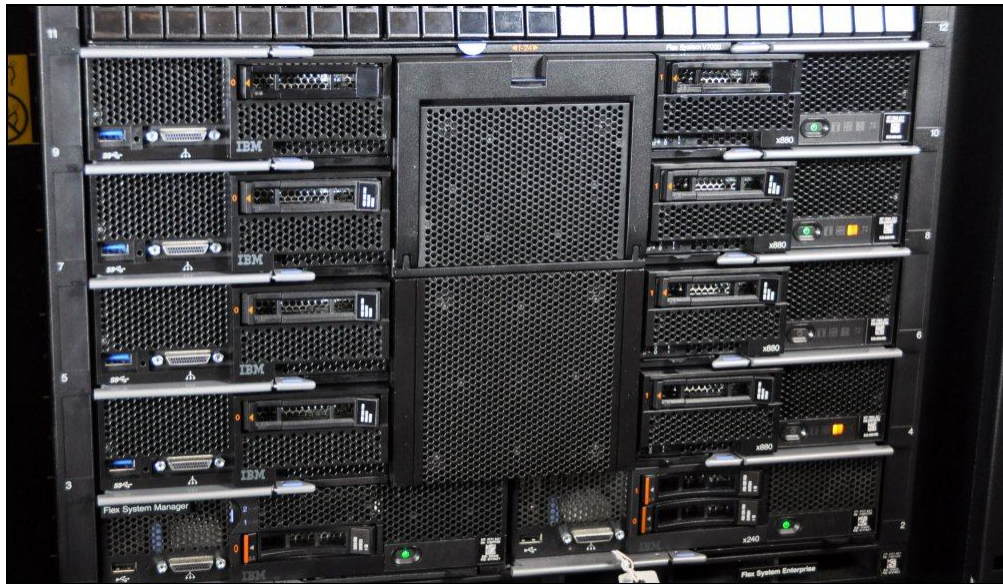
Figure 5. Four x880 X6 Compute Nodes as an 8-socket complex that is installed in a Flex System Enterprise Chassis
