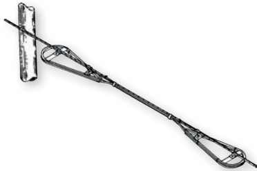
Reserve Cable Storage
