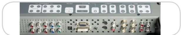
Multiple video inputs (VGA, DVI, dual BNC, S-Video and Component) allow for effortless system integration
