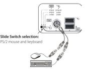
PS/2 Keyboard and USB Mouse: Slide switch to the center position
