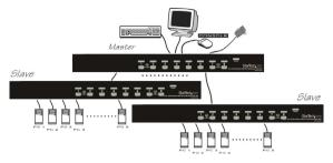
The maximum number of computers controlled in a Master/Slave configuration with all 16-port units is 136, with 8 units of 16-port Slaves (to PC 1 - PC 8) and each Slave connected to 16 computers, plus 8 more computers connected directly to the Master (to ports PC A - PC H):
