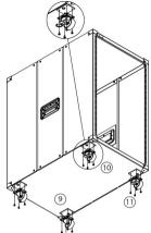
**Warning!** To prevent bodily injury, please make sure that the rack is installed in a structurally sound environment with a level floor, and that all of the hardware has been assembled securely and checked for stability before loading equipment. When installing equipment into the rack, start from the bottom of the rack first and move upwards, keeping the heaviest equipment at the bottom to avoid a situation where the rack becomes top heavy.
