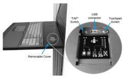
Two switches are also hidden in this compartment, that can assist with the use of an external mouse. The Touchpad switch can disable the touchpad completely, or simply disable the touchpad scrolling feature. While the "Tap" switch can disable the touchpad "Tap" feature, so tapping the touchpad does not register as a mouse-click.
