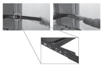
4. Attach the extensions brackets to both sides of the KVM switch module. Please note the length of the extensions and mount them as shown.
