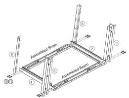
Using the remaining two Beams assembled in step 1, line up the other set of Left and Right Vertical Rails and fasten them to the Base and Top Brackets as shown.
