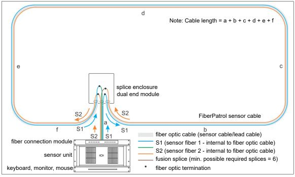
Figure 14 FiberPatrol fully closed redundant loop configuration
