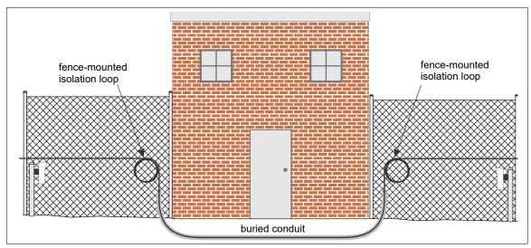
Figure 37 Perimeter structure bypass (below ground)
