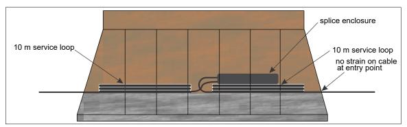
Figure 69: Buried sensor cable splice recommendations
