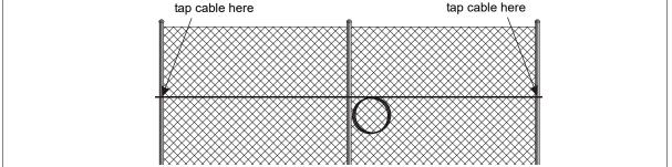
Figure 107 Tap test location - service loops
