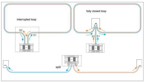
Figure 86 FiberPatrol sensor cable configurations
