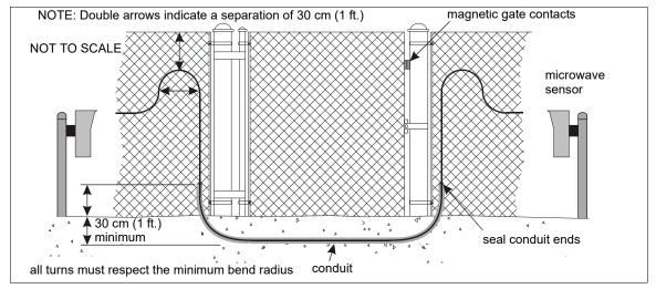
Figure 23 Gate bypass
