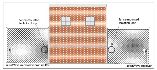
Figure 35 Perimeter structure bypass (through structure)
