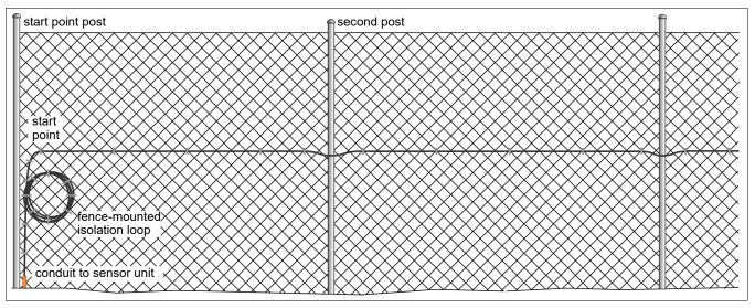
Figure 58 Cable installation procedure
