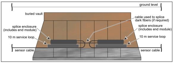
Figure 45 Back-to-back end module installation
