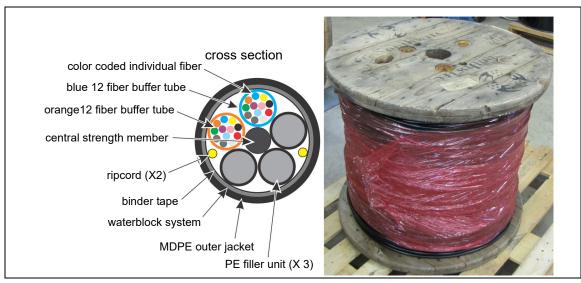
Figure 9 FiberPatrol sensor cable/non-detecting lead cable
