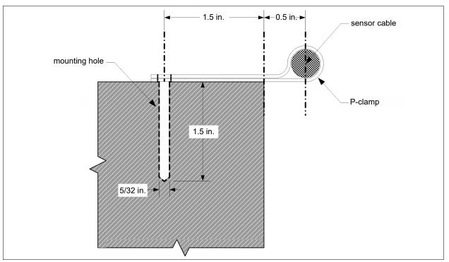
Figure 60 Masonry surface mounting hole dimensions
