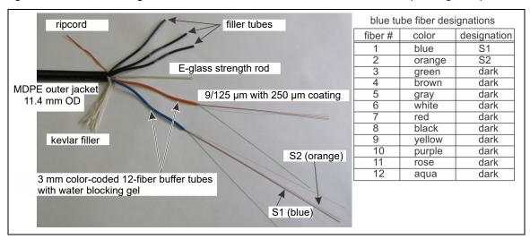
Figure 7 FiberPatrol standard sensor cable (FPSP0424)
