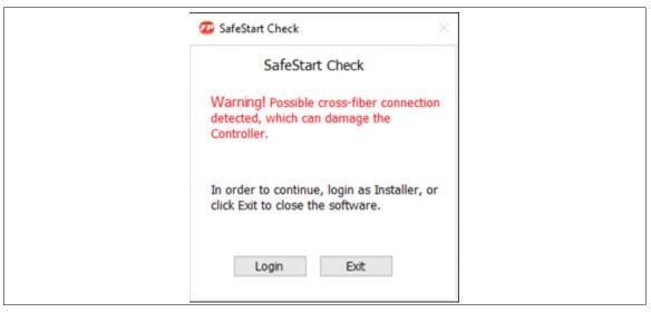
Figure 80 FiberPatrol Safe Start Warning
