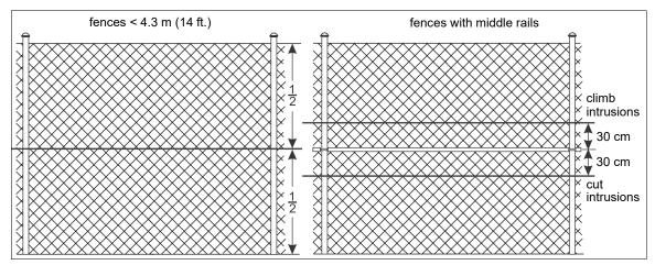
Figure 20 Recommended fence height/cable pass configurations
