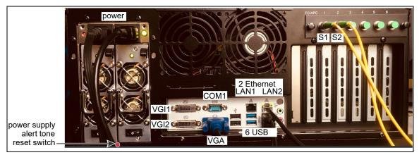
Figure 3 FiberPatrol sensor unit rear view
