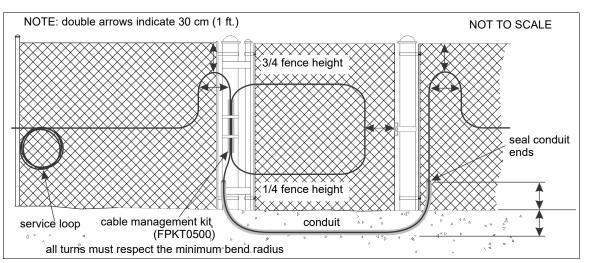
Figure 24 Cable layout on a single panel swinging gate
