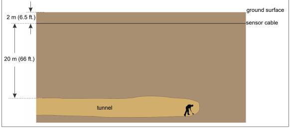
Figure 64: Sensor cable burial for tunneling detection
