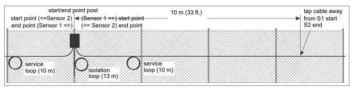
Figure 91 Tap test location - Set Start Sensor 1 (fully closed loop example)
