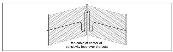
Figure 101 Tap test location - at corners or heavy gauge posts
