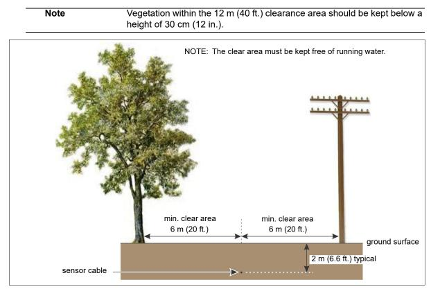
Figure 65: Minimum separation distances from obstacles
