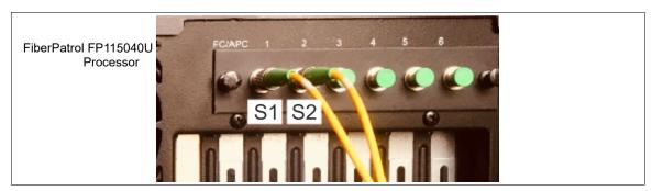
Figure 74 FP115040U fiber connections
