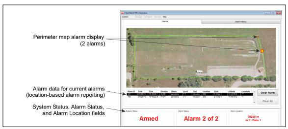
Figure 137 Operator Alarms panel (2 alarms)
