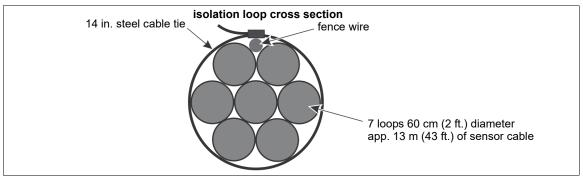
Figure 33 Isolation loop (fence-mounted)
