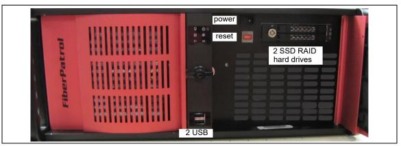
Figure 2 FiberPatrol sensor unit front view
