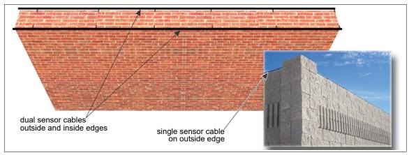
Figure 29 Protecting a masonry structure along the perimeter
