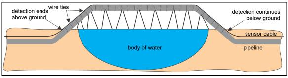
Figure 47 Sensor cable bypass (body of water)
