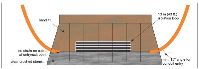
Figure 55: Buried vault isolation loop recommendations
