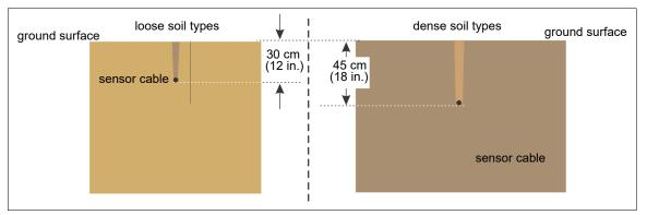
Figure 63: Sensor cable burial for intrusion detection
