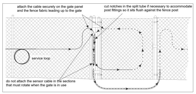
Figure 59 Cable installation on gates
