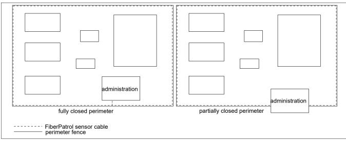
Figure 11 FiberPatrol example fully closed & partially closed configurations
