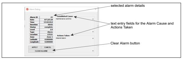
Figure 140 FiberPatrol Alarm Dialog
