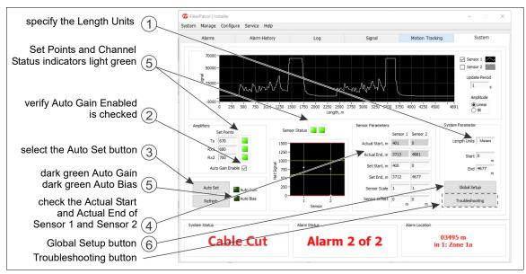
Figure 87 FiberPatrol System configuration (installer access level)
