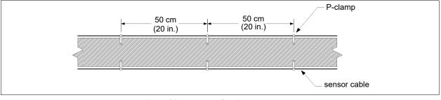
Figure 61 Masonry surface P-clamp spacing
