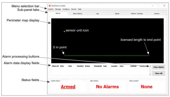
When first started, the sensor unit loads a default Alarm Screen configuration with a straight line perimeter, in which the cable length is based on the license limit.
