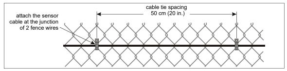
Figure 49 Cable tie spacing on fence fabric
