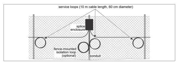
Figure 42 Cable splice service loops and fence-mounted isolation loop at fully closed perimeter start/end point
