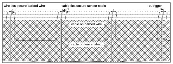
Figure 21 Sensor cable installation on barbed wire fence
