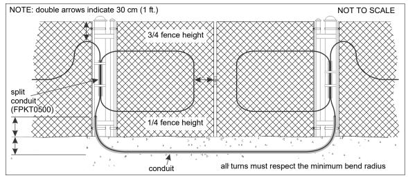
Figure 25 Double panel swinging gate
