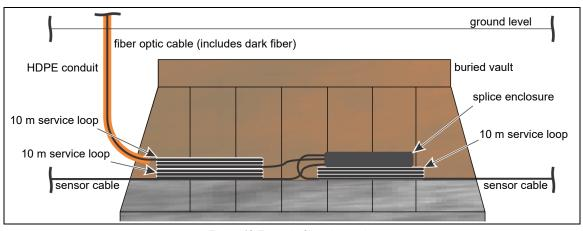
Figure 43 Example fiber drop point
