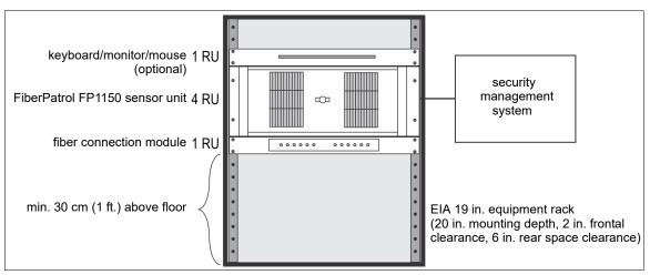
Figure 71 FiberPatrol equipment room block diagram
