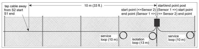
Figure 93 Tap test location - Set Start Sensor 2 (fully closed loop example)
