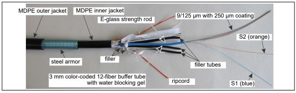
Figure 8 FiberPatrol armored sensor cable (FPSP0624)
