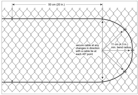
For all cable turns attach the cable to the fence fabric at each 45° point of the curve.
