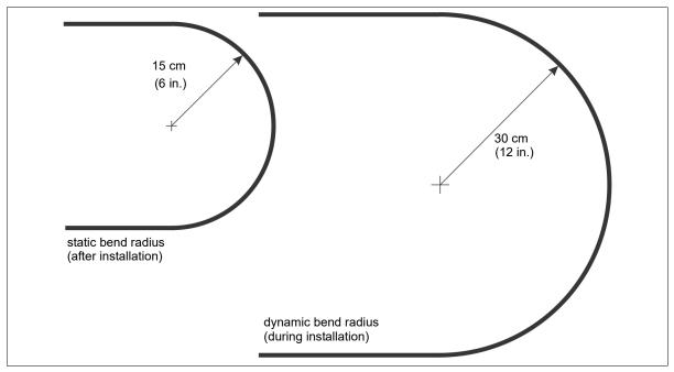
Figure 66: Smallest allowable bend radius (sensor cable)
