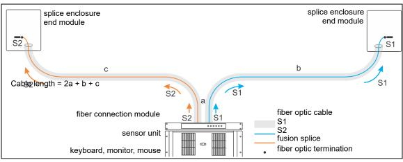
Figure 17 FiberPatrol split configuration (2 lead cables)
