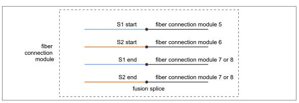
Figure 72 Sensor cable fiber splicing connections
