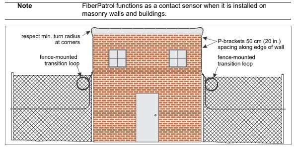
Figure 28 Protecting a masonry structure along the perimeter
