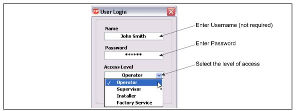
Figure 135 FiberPatrol login window
