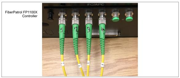
Figure 75 FP115040H fiber connections (1 - 4)
