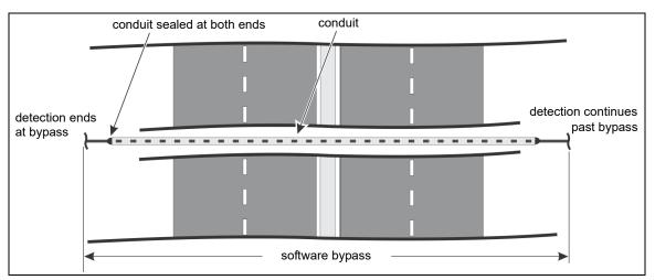
Figure 46 Sensor cable bypass (road crossing)
