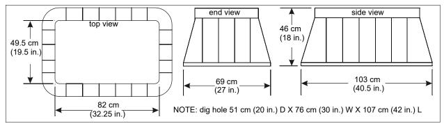
Figure 10 Buried vault dimensions
