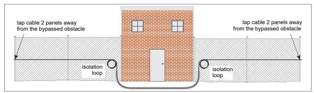
Figure 105 Tap test location - bypassed obstacles
