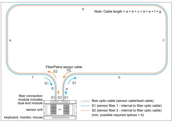
Figure 15 FiberPatrol partially closed redundant loop configuration
