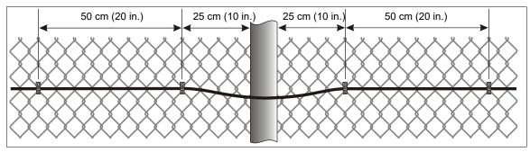
Figure 50 Cable tie spacing at fence posts
