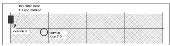
Figure 96 Tap test location - Set Start (Split configuration)
