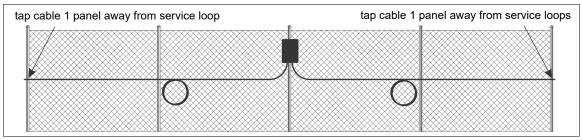
Figure 100 Tap test location - outdoor splices
