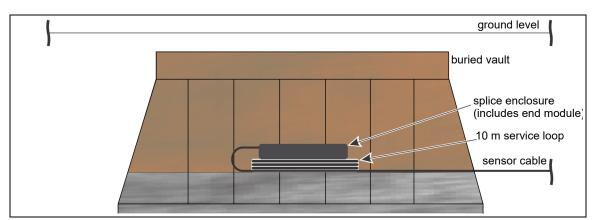
Figure 44 Single end module installation
