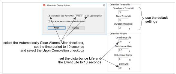
Figure 90 Temporary settings for location calibration
