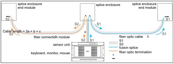
Figure 16 FiberPatrol split configuration (1 lead cable)
