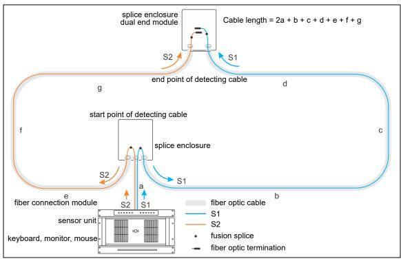
Figure 18 FiberPatrol split configuration (closed loop with start point splice)
