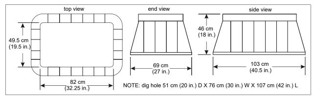
Figure 68: Buried vault dimensions
