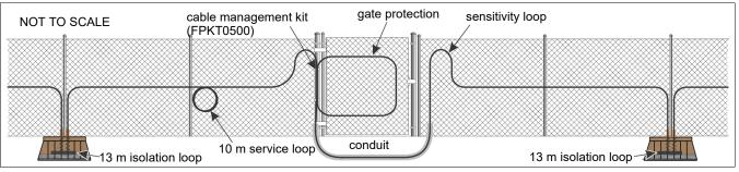
Figure 27 Independent gate zone (with buried isolation loops)
