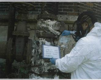
Site Name: M&H Zinc TDD#: S05-0808-001 Location: Lassalle, Illinois Date: 08/26/08 Direction: East Photographer: T. Koach Description: Sample MH-10, pipe insulation from an elbow on the ESE side of Rolling Mill.
