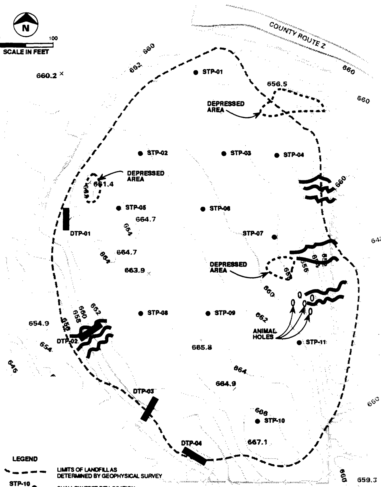
FIGURE C-7 SIGNIFICANT VISIBLE CAP DAMAGE ONALASKA LANDFILL RI
