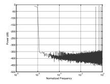
Fig. 7: PSD of MASH 1-1-1 with n=19 and input =2<sup>n</sup>/2
