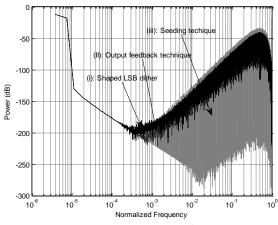
Fig. 8: PSD of a third order SQ\_EFM with n=13 and input =2<sup>n</sup>/2. The FFT length NFFT=2<sup>18</sup>; (i) Shaped LSB dither, (ii) Output feedback technique and (iii) Seeding technique
