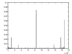
Fig. 9: Autocorrelation function of quantization error of a SQ\_EFM with n=19 bit and input=2<sup>n</sup>/2
