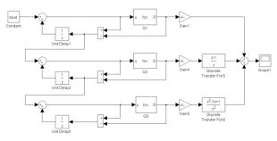
Fig. 3: Block diagram of MASH 1-1-1
