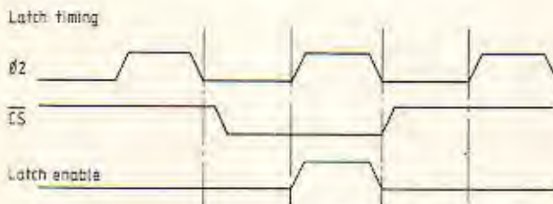
Fig. 8. Enable signal and latch timing for the d-to-a converter.
