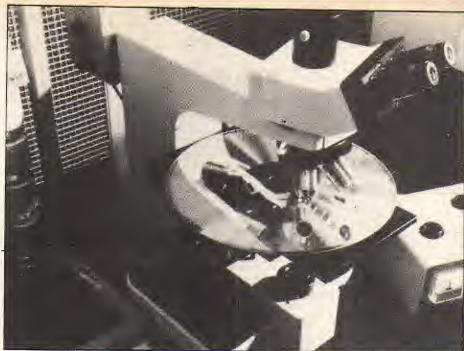
A LaserVision disc at a visual inspection station at the Blackburn disc-pressing plant. Discs are produced under 'clean room' conditions like those needed for integrated circuit production.
