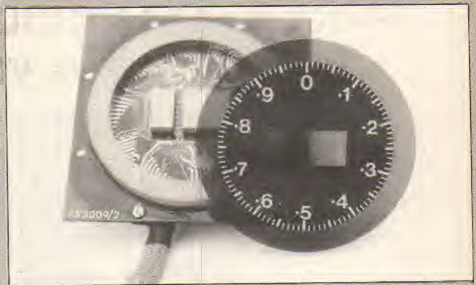
When Racal-Decca bought some digital displays from Hewlett-Packard for use in radar equipment, the dials incorporated in the displays were manufactured by Chequers (UK) Ltd in London, some 15 miles away from the Racal-Decca Marine Radar plant in New Malden, Surrey. To cover those 15 miles they had in fact travelled 10,000 miles across the Atlantic and back. The dials have an outer ring of 100 l.e.ds to give an analogue readout with three seven-segment l.e.d. digits in the centre. Because the printed dial has to match up with the l.e.ds, the diodes are positioned and the printing registered to within 0.003in.
