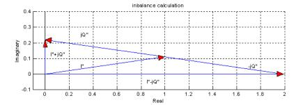
Fig. 106 Modulation error: I/Q imbalance
