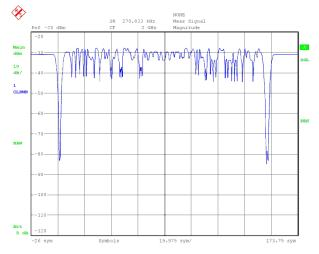
Fig. 18 Meas. 4: EDGE demodulator, correct demodulation
