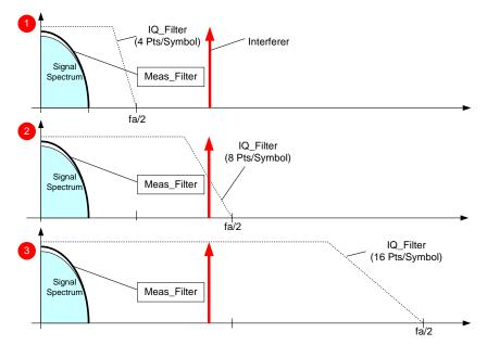
Fig. 27 Selected oversampling rates (I/Q bandwidth, interference)
