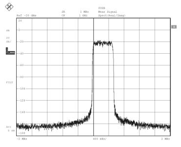
Fig. 80 Spectrum of measurement signal 8VSB (pilot carrier always removed) 8VSB (ATSC)
