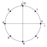
Fig. 43 Symbol mapping – 8PSK / NATURAL
