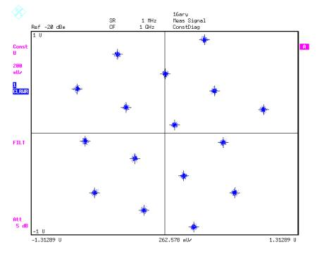
Fig. 77 Demodulation of a 16ary USER-QAM
