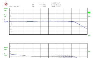
Fig. 255 Possible AM/PM conversion diagram with overdrive condition
