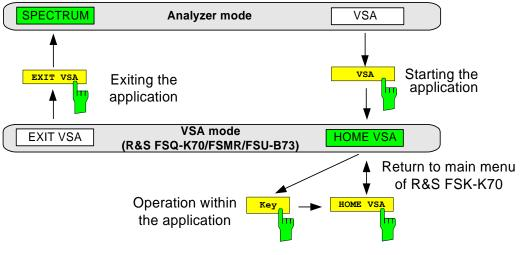
Fig. 4 Overview: calling and ex iting option FSQ-K70/FSMR/FSU-B73
