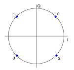
Fig. 60 Logical symbol mapping – OQPSK / CDMA2K\_REV
