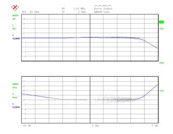
Fig. 256 Possible AM/PM conversion diagram with overdrive condition
