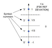
Fig. 62 Symbol mapping – 4-FSK / NATURAL
