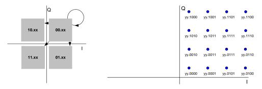
Fig. 74 Symbol mapping D64 QAM / DVB-C
