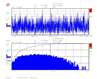
Fig. 120 Result display split screen *EVM* (upper diagram) *ERROR STATISTIC* + *EVM* (lower diagram)
