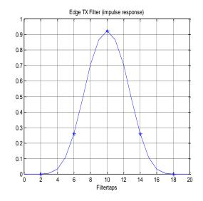
Fig. 48 EDGE TX filter
