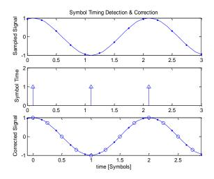
Fig. 86 Symbol timing detection & correction
