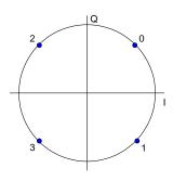
Fig. 42 Symbol mapping – QPSK / CDMA2K\_FWD
