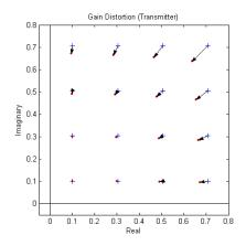
Fig. 107 Nonlinear distortions: amplitude distortion (transmitter)
