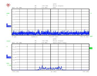
Fig. 248 Displayed error spectrum with correct filter settings
