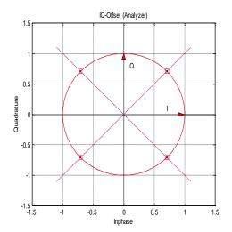
Fig. 101 Modulation error: compensation of origin offset
