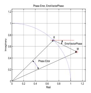
Fig. 99 Modulation error: EVM, magnitude error
