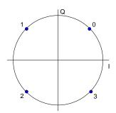
Fig. 41 Symbol mapping – QPSK / NATURAL
