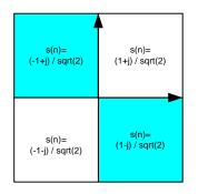
$$\begin{cases} 0 \le \arg(x(n)) < \frac{\pi}{2} & \to \quad s(n) = \frac{1}{\sqrt{2}} (1+j) \\ 1\frac{\pi}{2} \le \arg(x(n)) < 2\frac{\pi}{2} & \to \quad s(n) = \frac{1}{\sqrt{2}} (-1+j) \\ 2\frac{\pi}{2} \le \arg(x(n)) < 3\frac{\pi}{2} & \to \quad s(n) = \frac{1}{\sqrt{2}} (-1-j) \\ 3\frac{\pi}{2} \le \arg(x(n)) < 4\frac{\pi}{2} & \to \quad s(n) = \frac{1}{\sqrt{2}} (1-j) \end{cases}$$
