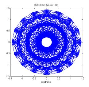
Fig. 49 Vector diagram: transmitted EDGE signal
