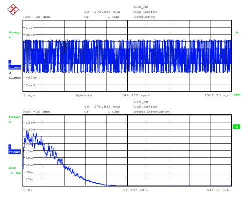
Fig. 202 Result display CAPTURE BUFFER FREQUENCY (upper diagram) Result display SPECTRUM -> CAPTURE BUFFER FREQUENCY (lower diagram)
