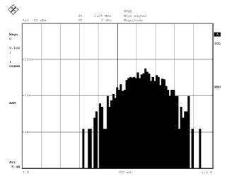
Fig. 253 Statistical distribution of magnitude error in the event of underdrive
