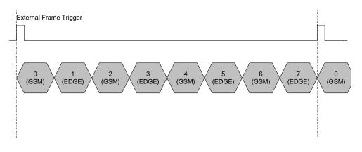
The transmitter settings cause bursts in time slots 1 to 7. GSM and EDGE bursts are transmitted alternately.
