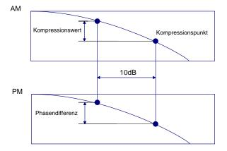
The compression value is set with CALC:MARK:FUNC:CPO:VAL. The compression point is queried with CALC:MARK:FUNC:CPO:POW?. The phase difference is queried with CALC:MARK:FUNC:CPO:PHD?.
