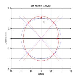
Fig. 103 Modulation error: gain imbalance (analyzer)
