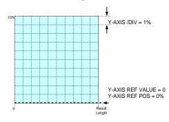
Fig. 226 Example of RANGE, time display (EVM lin)
