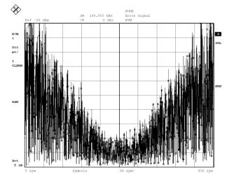
Fig. 243 Displayed EVM with incorrect setting of the symbol rate
