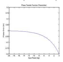
Fig. 113 Nonlinear distortions: phase distortion (transmitter)
