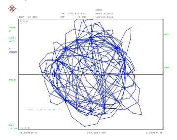
*RAW* For further applications (e.g. distortion measurement on transmitter output stages), demodulated but unfiltered measurement signals that are not falsified by filtering in the receiver are required.
