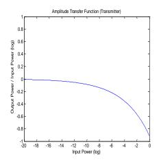
Fig. 109 Amplitude transfer function (transmitter)
