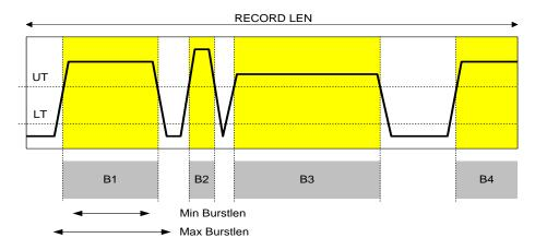
Fig. 84 Record buffer containing several bursts
