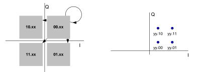
Fig. 72 Symbol mapping D16 QAM / DVB-C
