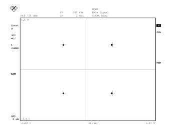
Fig. 244 Constellation diagram with correct setting of the symbol rate
