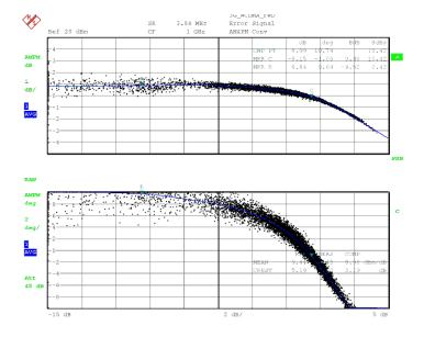
Fig. 184 AM & PM CONVERSION result display (AM-AM upper diagram, AM-PM lower diagram)
