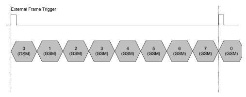
The transmitter settings cause GSM bursts in time slots 0 to 7.
