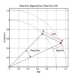
Fig. 98 Modulation error: EVM, magnitude error
