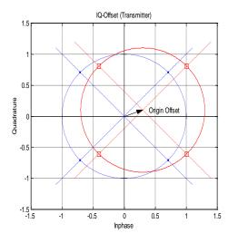
Fig. 100 Modulation error: origin offset (I/Q offset)
