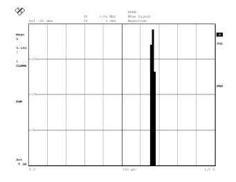
Fig. 252 Statistical distribution of magnitude error with correct modulation
