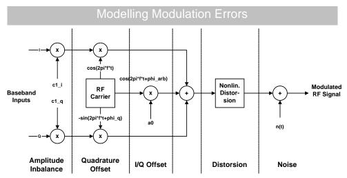
Fig. 96 The following error model is used for the examples below:
