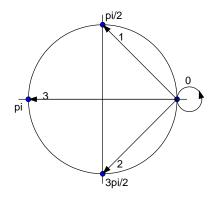
Fig. 54 Logical mapping – (NADC, PDC, PHS, TETRA)
