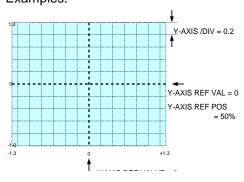
Fig. 225 Example of RANGE, I/Q display X AXIS/DIV is used together with Y AXIS/DIV
