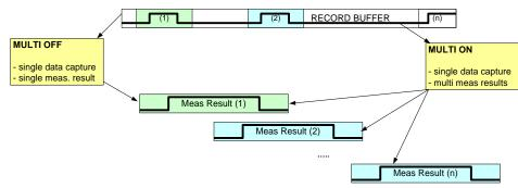
Fig. 131 MULTI ON/MULTI OFF: Multiple measurement evaluations per data capture
