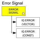
For softkeys that offer more than one setting, the softkey labelling indicates the current setting. For example, the following settings are possible for the measurement evaluation IQ Error:
