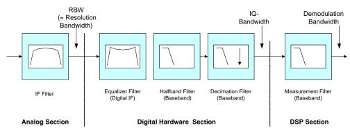
Fig. 26 Block diagram of bandwidth-relevant filters for vector signal analysis
