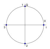
Fig. 40 Symbol mapping – QPSK / WCDMA
