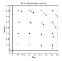
Fig. 111 Nonlinear distortions: phase distortion (transmitter)
