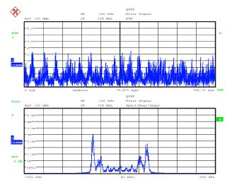
Fig. 249 Displayed error spectrum with different filter settings
