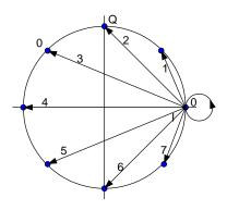
Fig. 53 Physical constellation diagram – D8PSK / NATURAL
