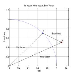
Fig. 97 Modulation error: error vector
