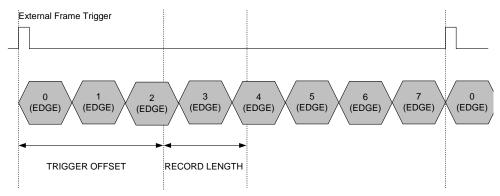
The transmitter settings cause EDGE bursts in time slots 0 to 7.
