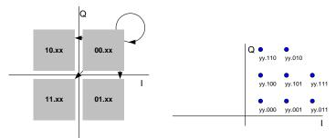
Fig. 73 Symbol mapping D32 QAM / DVB-C
