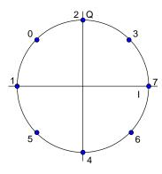
Fig. 46 Logical symbol mapping - 3pi/8-8PSK / EDGE
