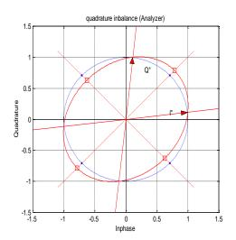
Fig. 105 Modulation error: quadrature imbalance (analyzer)
