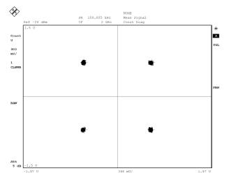
Fig. 245 Constellation diagram with incorrect setting of the symbol rate
