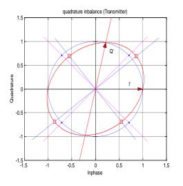
Fig. 104 Modulation error: quadrature imbalance (transmitter)
