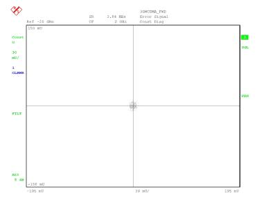
Fig. 187 IQ ERROR result display (constellation diagram)
