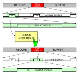
Fig. 134 DEMOD NEXT RIGHT Burst signal, demodulation of the next burst signal
