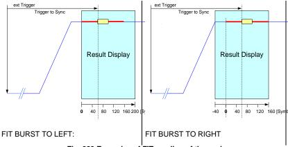
Fig. 223 Examples of FIT: scaling of time axis
