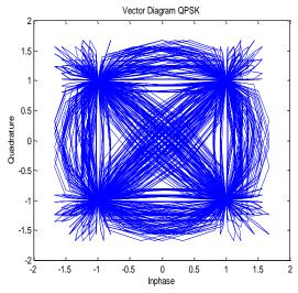
Fig. 58 PSK vector diagram with alpha = 0.35
