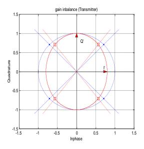
Fig. 102 Modulation error: gain imbalance (transmitter)
