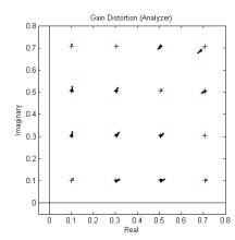
Fig. 108 Amplitude distortion (analyzer)
