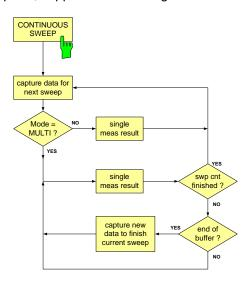
Fig. 138 COUNTINUOUS SWEEP: Automatic data capture
