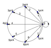
Fig. 52 Logical symbol mapping – D8PSK / NATURAL
