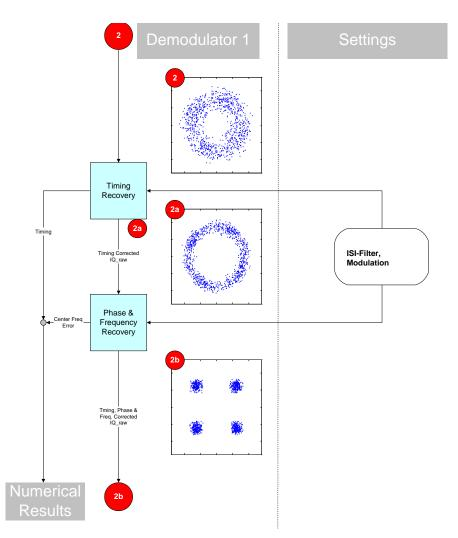
Fig. 85 IQ-Demodulator: Timing, Phase, Frequency Recovery
