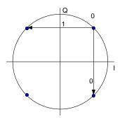
Fig. 64 Physical constellation diagram – MSK
