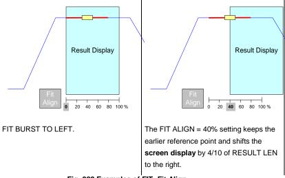
Fig. 222 Examples of FIT: Fit Align
