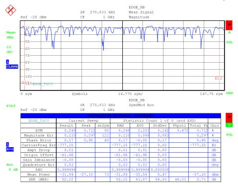
Fig. 122 Measurement window of the R&S FSQ-K70/FSMR-B73/FSU-B73 option
