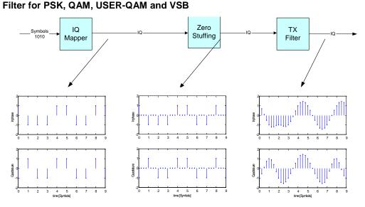
Fig. 31 Generation of baseband transmit signal (PSK, QAM, USER-QAM and VSB)
