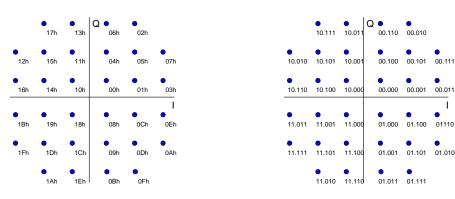
Fig. 68 Symbol mapping – 32QAM / DVB-C
