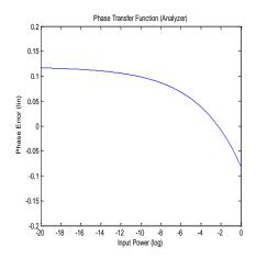
Fig. 114 Phase distortions (analyzer)
