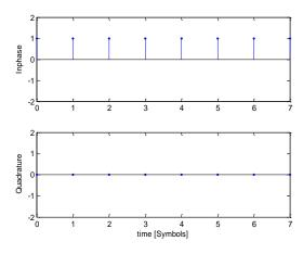
Fig. 44 I/Q symbol stream before 3pi/8 rotation
