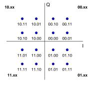
Fig. 67 Symbol mapping – 16QAM / DVB-C
