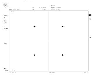
Fig. 250 Constellation diagram with correct modulation
