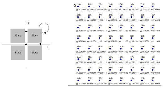
Fig. 76 Symbol mapping D256 QAM / DVB-C
