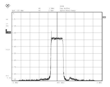
Fig. 79 8VSB spectrum at the input of the analyzer (pilot carrier visible to the left)
