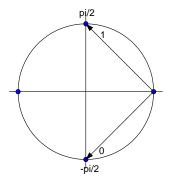
Fig. 63 Logical symbol mapping – MSK / NATURAL
