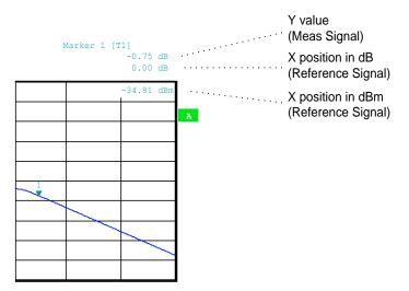
Fig. 185 AM & PM CONVERSION result display, marker field)
