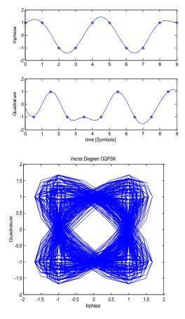
Fig. 59 OQPSK vector diagram with alpha = 0.35
