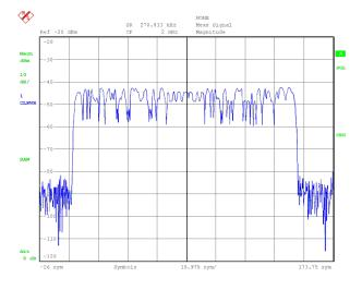
Fig. 17 Meas. 3: Burst search, manual level setting
