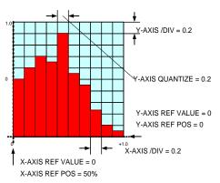
Fig. 228 Example of RANGE, statistical display Quantize
