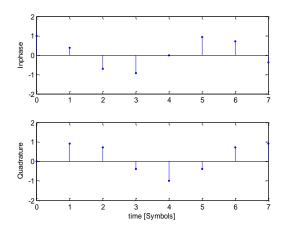
Fig. 45 IQ-I/Q symbol stream after 3pi/8 rotation
