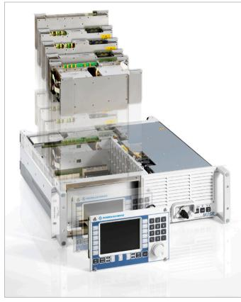
Modular radio design, for easy upgrades, scalability and easy maintenance.
