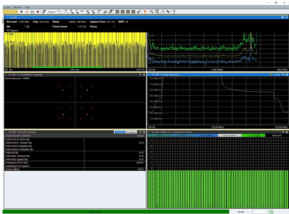
Fig. 3-8: Measurement Results of the 5G NR FR2 uplink signal at 26 GHz on the VSE
