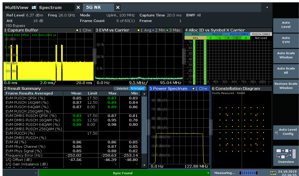
Fig. 4-28: Signal quality Measurement results of 5G NR TDD UL signal at 26GHz
