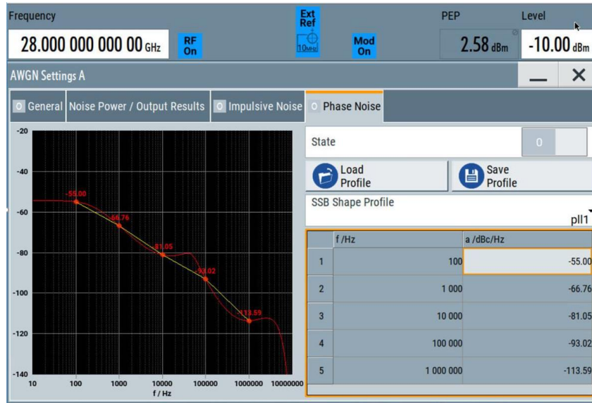
Fig. 4-4: Phase noise configuration on the SMW
