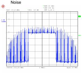
Fig. 15 Noise floor at 46 dB of DVB-T spectrum with superposed impulsive noise and extended dynamic range
