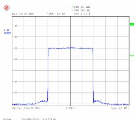
Fig. 11 Noise floor at 50 dB of test transmitter's DVB-T spectrum
