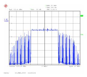
Fig. 13 Noise floor at 50 dB of DVB-T spectrum with superposed impulsive noise (max.power) at 50 dB
