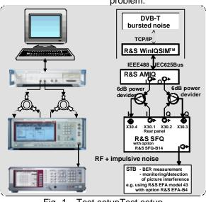
Fig. 1 Test setupTest setup
