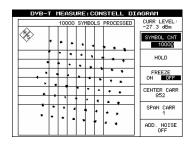
Fig. 3a Constellation diagram of central suppression.
