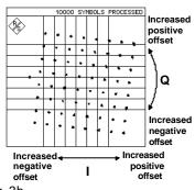
Coarse adjustment is performed by carrier in 2k mode prior to rotating the constellation diagram (by adjustment of residual carrier varying the offset of the Q component) and by shifting the I/Q value pairs (by varying the offset of the I component).
