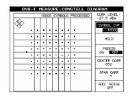
Fig. 3c Nearly constellation correct diagram of central carrier in 2k mode with coarsely adjusted residual carrier suppression.
