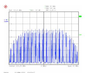
Fig. 12 Example: spectrum of impulsive noise at max. power
