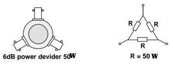
Fig. 2  $\,$  50  $\Omega$ , 6 dB power divider; mechanical design and schematic diagram
