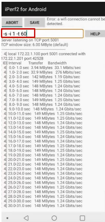
Figure 57 iPerf command on DUT (Server, TCP) and measurement result
