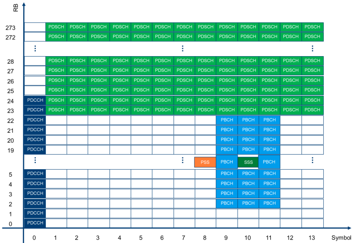
Figure 11 Resource allocation of Slot 0 (symbol 0 is reserved for PDCCH) 3
