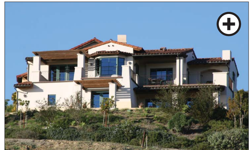
The same Alta Vista neighborhood home viewed from the front of the house. Setting the house into the hillside reduces the apparent height. (28.1, 29.1, 29.2)
