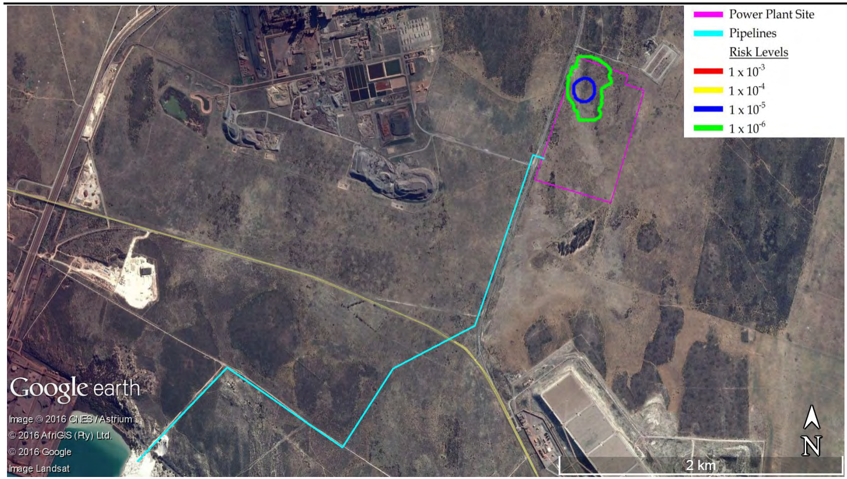
Figure 10.19 Risk Contours for Individual Risk of Fatality for Saldanha Steel Propane Storage Facility during the Second Year of Construction – Persons Located Indoors
