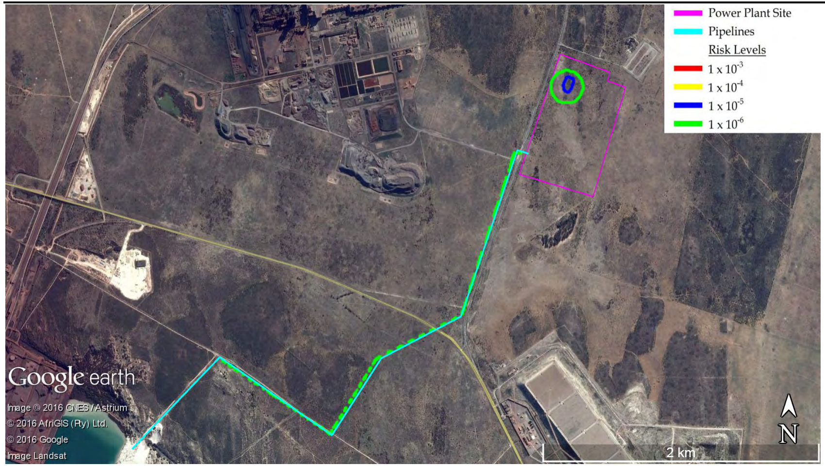
Figure 10.25 Risk Contours for Individual Risk of Fatality for Saldanha Steel Natural Gas Pipelines and Propane Developments during Normal Operation – Persons Located Indoors
