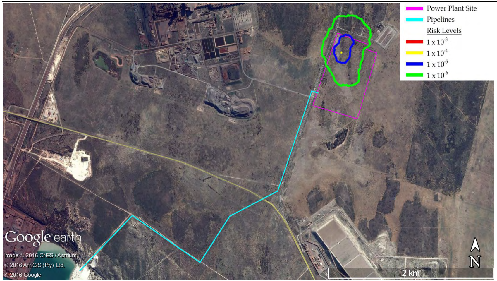
Figure 10.18 Contours for Individual Risk of Fatality for Saldanha Steel Propane Storage Facility during the Second Year of Construction – Persons Located Outdoors
