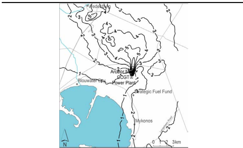
Figure 10.4 99th percentile of the predicted 1-hour CO concentrations ( \mu\text{g}/\text{m}^3 ) resulting from emissions from ArcelorMittal CCGT power plant (operation)
