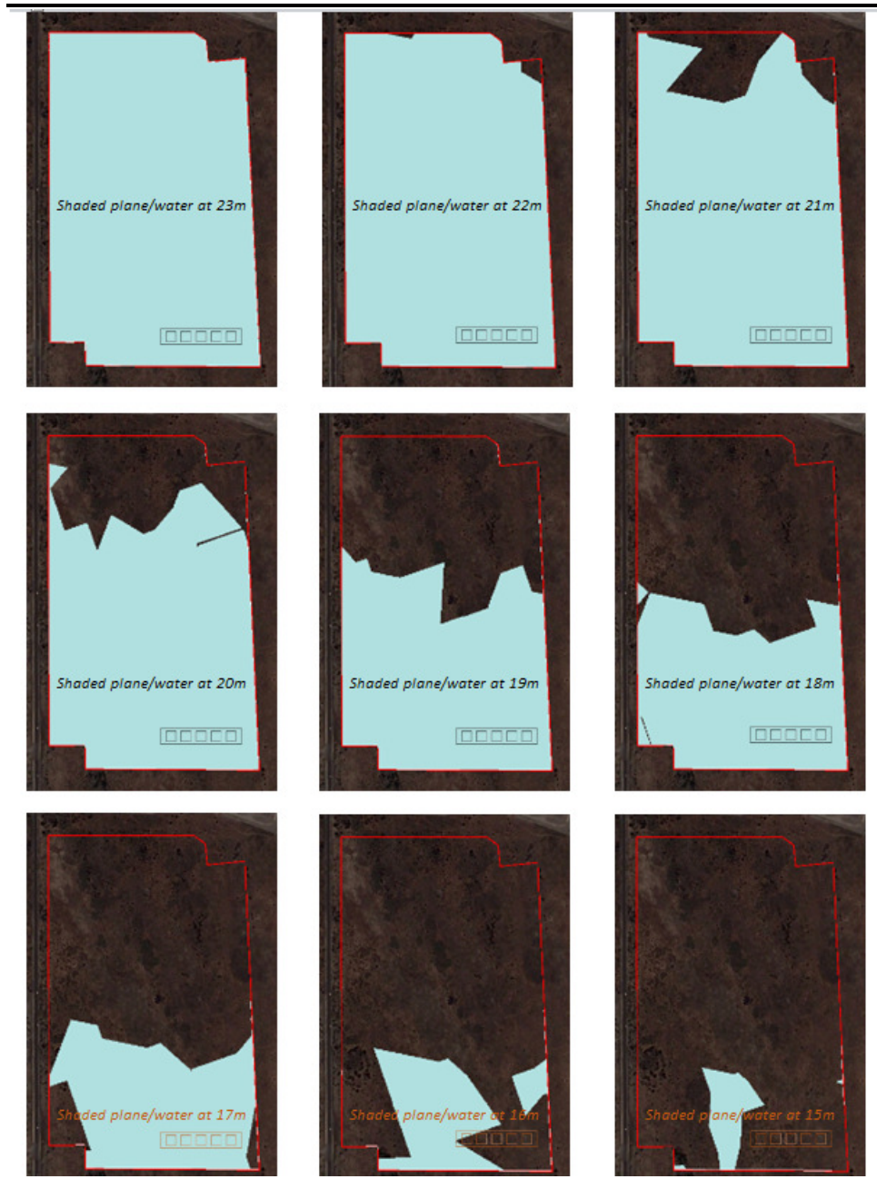
Figure 3.17 Surface Water Drainage
