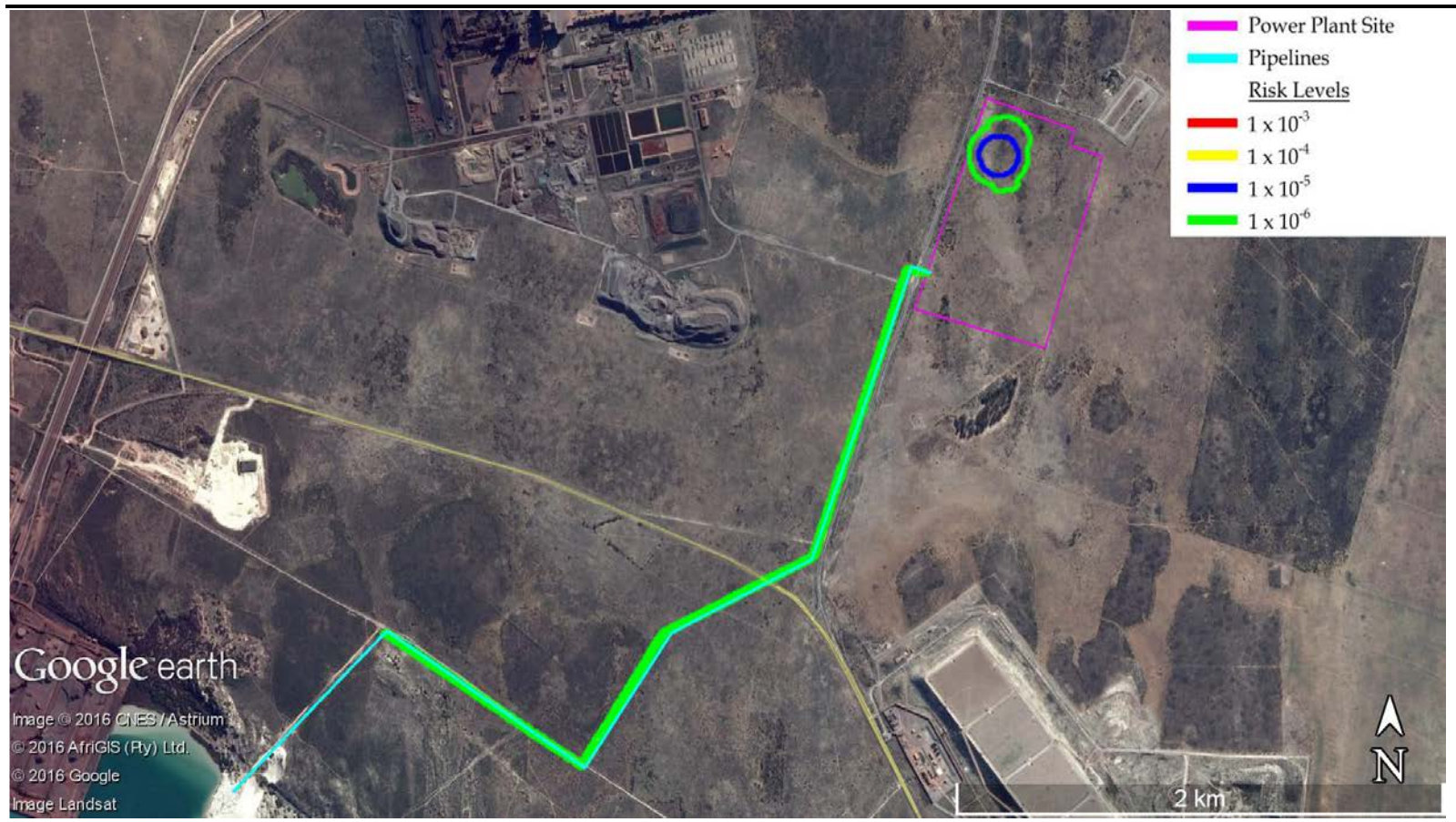
Figure 10.24 Risk Contours for Individual Risk of Fatality for Saldanha Steel Natural Gas Pipelines and Propane Developments during Normal Operation – Persons Located Outdoors
