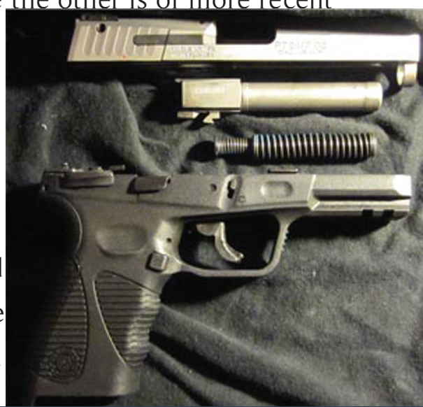
(A) The new Taurus 24/7 G2 is a compact, reliable 15+1 .40 S&W self-loading pistol. (B) The recoil spring is on a fulllength rod and the end of the barrel has a slight “cannon muzzle” to fit the slide. (C) One extra safety is the lever in the center of the trigger to prevent its travel unless it is first depressed. (D) The slide-to-frame fit is excellent and an ambidextrous thumb safety is also provided. (E) A loaded-chamber indicator is provided atop the slide. (F) Fixed 3-dot sights are provided and deliver a clear, strong sight picture.
