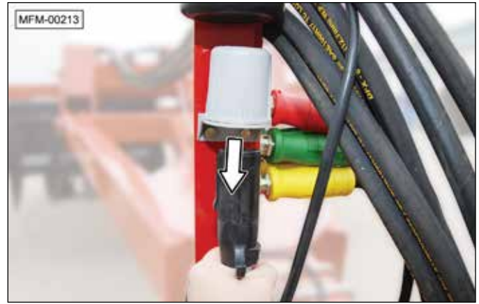
d. Connect the plug into the tractor's electrical socket.
