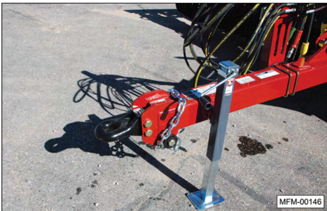
Transport lock secured in storage position.
