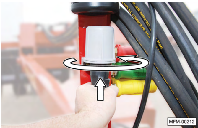
b. Push the plug upward and slightly rotate it again to release it from the socket.
