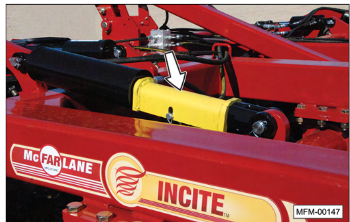
Transport lock secured over cylinder rod.
