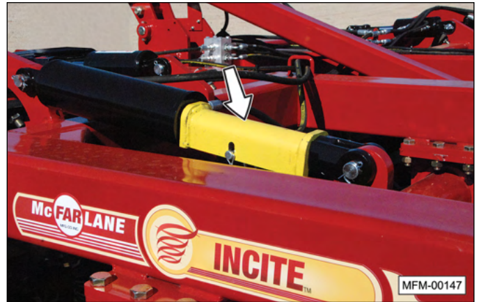
Transport lock secured over cylinder rod.
