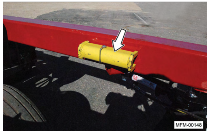
Transport lock secured in storage position.
