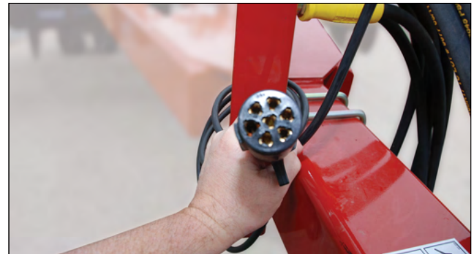
d. Connect the plug into the tractor's electrical socket.
