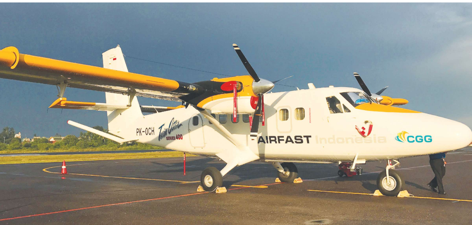
CGG Multi-Physics partnered with Airfast Indonesia and deployed its new sGrav meter with the Falcon AGG system on a modified Twin Otter aircraft to acquire its Falcon Full Spectrum Gravity survey in Sumatra. (Source: CGG Multi-Physics)
