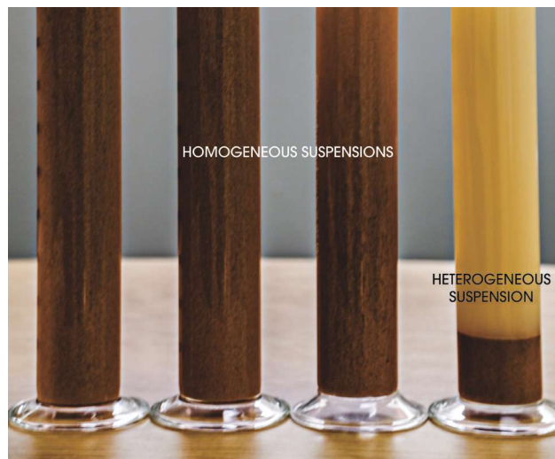
Binder Science’s proppant placement system keeps proppants in the homogenous flow regime. (Source: Binder Science)
