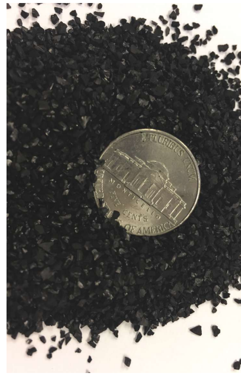
A solid particulate oil soluble chemical tracer is shown. (Source: Spectrum Tracer)
