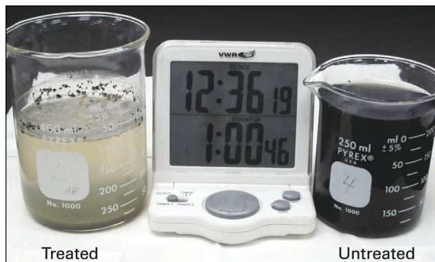
Figure 1. Before and after reaction of high-sulfide concentration produced water treated with peracetic acid.
