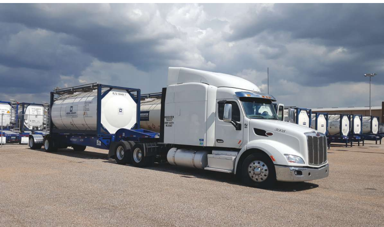
The ISO tanks are equipped with insulation, steam trace heating and cooling capabilities as well as optional safety features. (Source: Hoover Ferguson)
