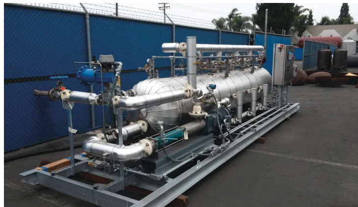
CoStrip is designed for degasification of water streams containing high loadings of oil and suspended solids. (Source: Veolia Water Technologies)
