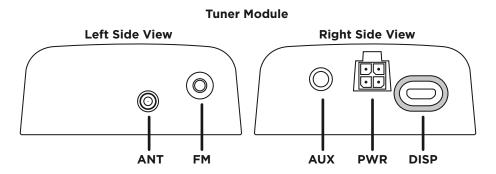
ANT (Antenna): Connection for the Magnetic Mount Antenna.
