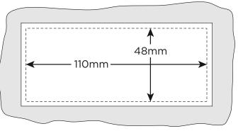
**3.** Once the opening has been cut, remove the template and place the Flush Mount in the opening. The Flush Mount is asymmetrical so the top/bottom orientation is not important.
