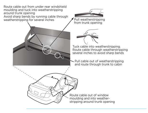
Bring cable out of weatherstripping and into trunk
