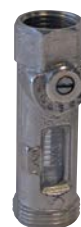
FLOW METER with Mechanical Regulation REF: FM 1234 BSP 1/2" (Female) - BSP 3/4" (Male) Hexagonal: SW19 Full Length: 81mm Flow capacity: 2 - 8 lt/min Temperature Range: +0°C - +100 °C Working Pressure: max 10 Bar Springs: Stainless Steel Indicator Plastic Seals: Buna
