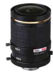
DH-PLZ20C0-P Dahua Lens 10,5-42mm • Formaat 1/1.7" • Aperture: F1.5 • Focus length: 10.5-42mm • Mount: CS
