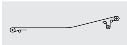
Fig.2.2 - Conveyor with horizontal belt with incline section, where the space permits a vertical curve and where the load requires the use of a single belt.
