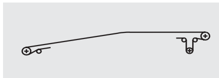
Fig.2.4 - Conveyor with horizontal and incline section where space does not allow a vertical curve and the load needs two belts to be employed.
