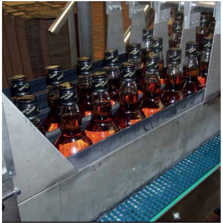
Conveyor with 500 belt.
