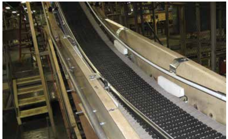
Conveyor with TCF7705 Belt
