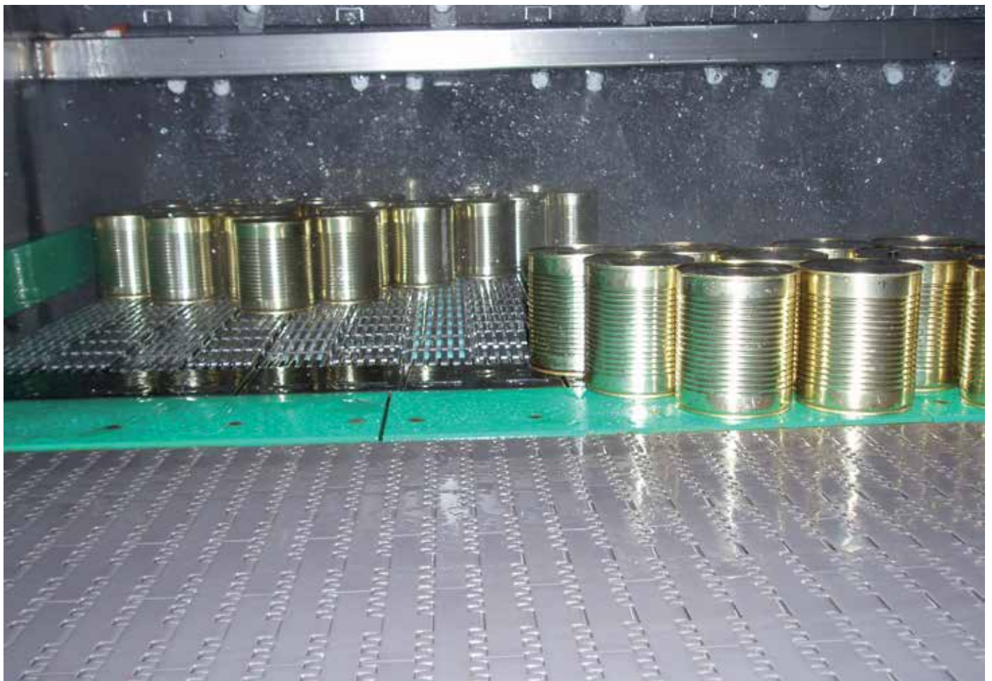
Fortrex 9227 belt in a food tunnel pasteurizer
