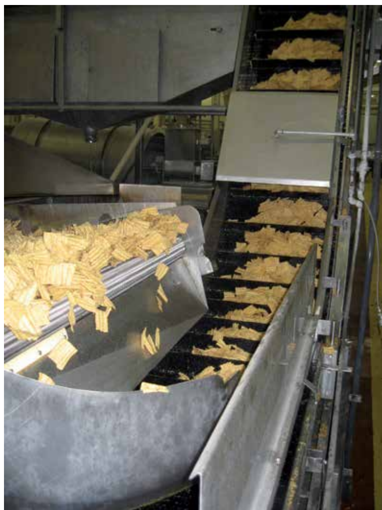
Inclined conveyor for chips fr2015 mattop chain
