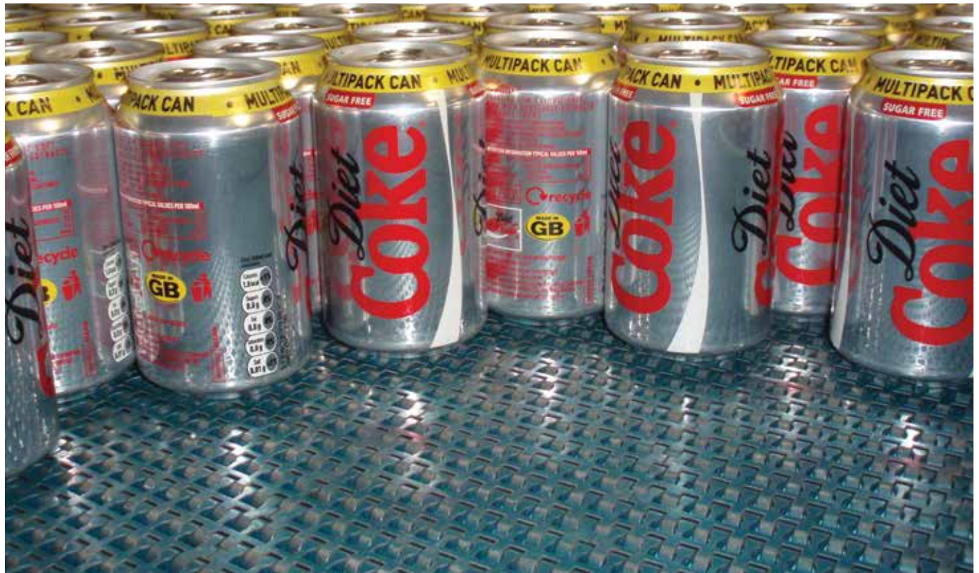
Conveyor with 500 belt.
