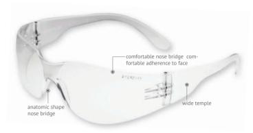
Lightweight modern universal spectacle with wide field of view. Provides protection against high speed particles (low energy impact V=45 m/s). Resistant to alkali and acid solutions.
