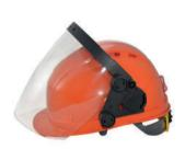
Unique **Slide** system of face shield locking assures maximum comfort and freedom of action, easy face shied transposition from one position to another. When there is no necessity of face protection, the visor might be easily lifted and locked. In working position the visor adheres to the helmet without gap, preventing hard particles ingress inside.
