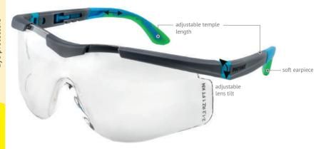
Light weighted modern universal spectacles with polycarbonate one-piece lens, water resistant double-sided hard/anti-fog coating. Reliable eye protection against high speed particles, abrasives, UV radiation. Provides protection against high velocity particles (low energy impact V=45 m/s). Resistant to alkali and acid solutions.
