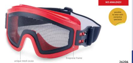
Protective goggles with ocular made of steel wire mesh (cell size 2 x 2 mm) painted with black enamel for rust prevention. Provides protection against high velocity particles.
