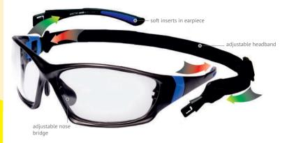
Model combines advantages of protective spectacles and goggles due adjustable headband. Panoramic one-piece lens, water resistant double-sided hard/anti-fog coating. Reliable eye protection against high speed particles, abrasives, UV radiation. Provides protection against high velocity particles (low energy impact V=45 m/s). Resistant to alkali and acid solutions. Additional frame for corrective lenses fixation.
