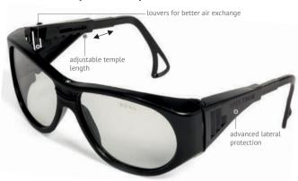
Universal protective spectacles providing protection against hard particles impact (0.5 J, V=5.1 m/s). Reliable plastic frame, widened temples with louvers for ventilation, temple length adjustment, lateral protection due widened temples, hardened mineral lenses.
