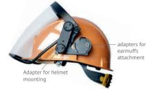
Model name: KBT VISION® ENERGO RX Item number: 04837 Visor: PC. clear Visor dimensions: 210 × 210 mm Working temperature range: from -50°C to +130°C Impact protection: 14.9 J Mass: 280 q
