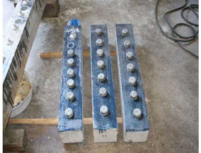
Figure 21: Discs Attached for the Pull-Off Test
