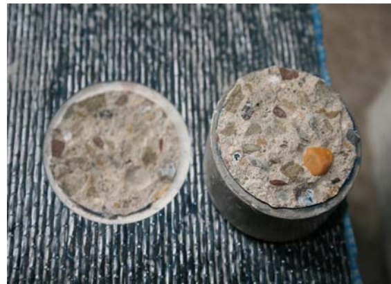
Figure 22: Testing of One Disc is in Progress Figure 23: Pull-Off Test Showing Cohesive Failure
