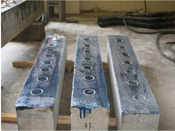
Figure 20: Field Prepared Prism Prepped for FRP Pull-Off Tests
