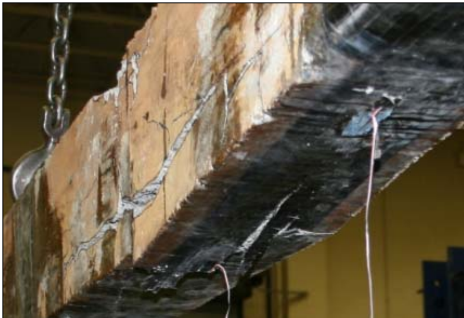
Figure 86: FRP rupture on CFO-repaired beam G-6
