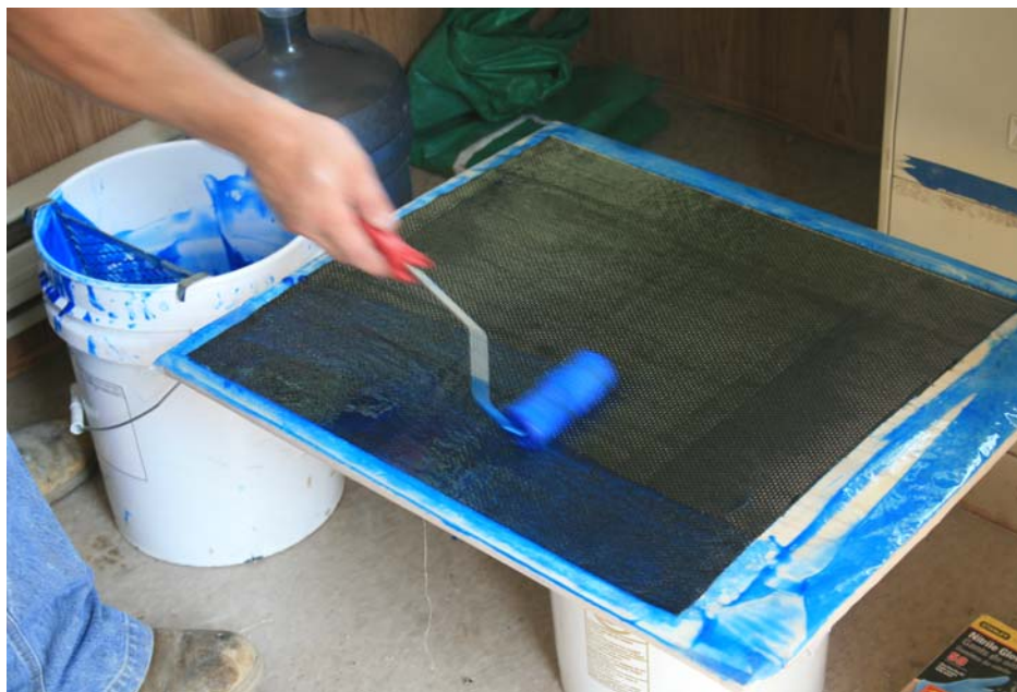
Figure 15: Fabrication of FRP Laminate to be used for Direct Tension Testing
