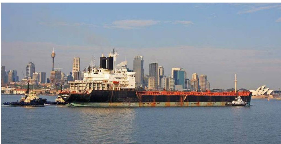
River Boyne on the way to Port Jackson, Sydney (Australia), November 2011. The coal bunkers can be seen behind the accommodation block. © Richard Goodman
