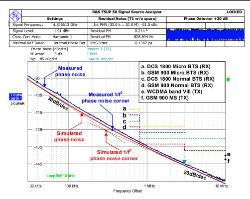
Figure 4.16: Measured (blue) and simulated (red) phase noise plots at 4.35 GHz,  $V_{\text{DD}}=1.3$  V and  $P_{\text{DC}}=41$  mW. Specifications (MS: mobile station, BTS: basestation) are normalized to the carrier frequency.
