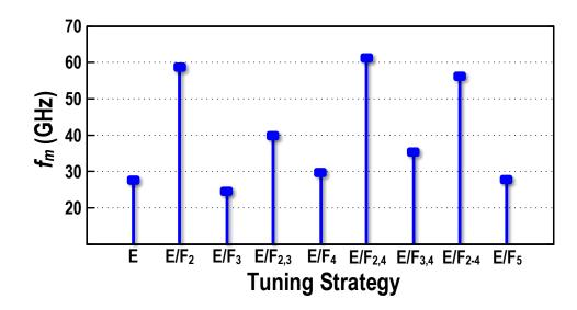
Figure 5.7: Maximum operating frequency of different flavors of class-E/F<sub>2</sub> PA. ( $\overline{R_{on}} = 850 \,\Omega\mu m$ ,  $\overline{C_{in}} = 1 \, fF/\mu m$ ,  $\overline{C_{out}} = 0.65 \, fF/\mu m$ ,  $\overline{I_{out}} = 0.6 \, mA/\mu m$ )
