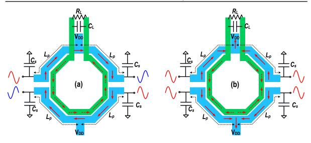
Figure 6.14: Transformer behavior in differential-mode (a) and common-mode (b) excitations.
