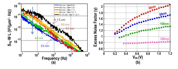
Figure 1.7: (a) Flicker noise scaling trend; (b) measured excess noise ( $\gamma$ ) factor versus drainsource voltage at 10 GHz and  $V_{gs} = 1.0$  V for different gate lengths of NMOS transistors in 40 nm LP technology [20].
