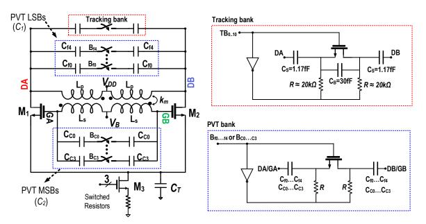
Figure 3.6: Schematic of the class-F DCO.
