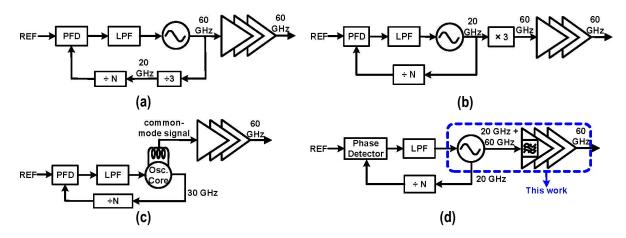
Figure 2.21: Evolution of the mm-wave PLL architecture (a): PLL with fundamental oscillator; (b): PLL with frequency multiplier; (c): PLL with push-push oscillator; (d): proposed PLL with harmonic boosting and extraction.
