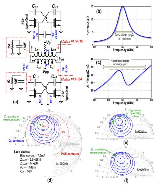
Figure 6.23: (a) simplified schematic of the driver amplifier; (b) real and (c) imaginary parts of the impedance seen at the input ports of the pre-driver matching network; constant  $G_p$  contours for  $2 \cdot 32 \cdot (1 \mu \text{m}/40 \text{nm})$  device at (d) 60 GHz, (e) 55 GHz and (f) 65 GHz.
