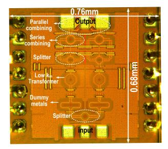
Figure 6.29: Chip micrograph.
