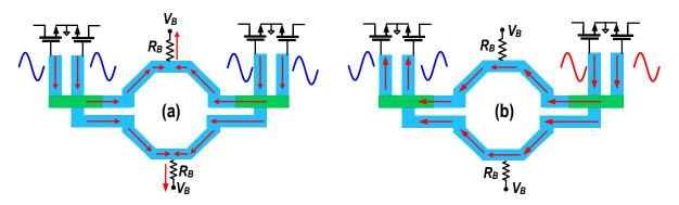
Figure 6.27: (a) Damping the undesired CM oscillation; (b) a combination of CM and DM oscillation.
