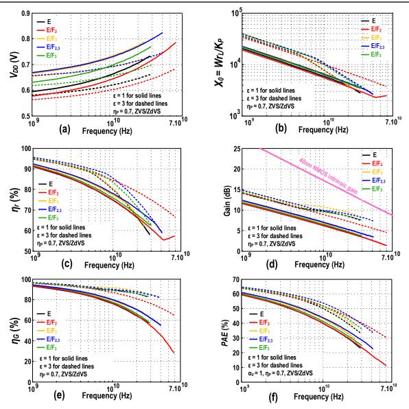
Figure 5.9: Characteristics of different flavors of class-E/F PA versus frequency at the maximum achievable PAE when taken  $V_{BK}$  into consideration. ( $\overline{R_{on}} = 850 \,\Omega\mu m$ ,  $\overline{C_{in}} = 1 \, fF/\mu m$ ,  $\overline{C_{out}} = 0.65 \, fF/\mu m$ ,  $\overline{I_{out}} = 0.6 \, mA/\mu m$ ,  $V_{BK} = 2 \,\mathrm{V}$ )
