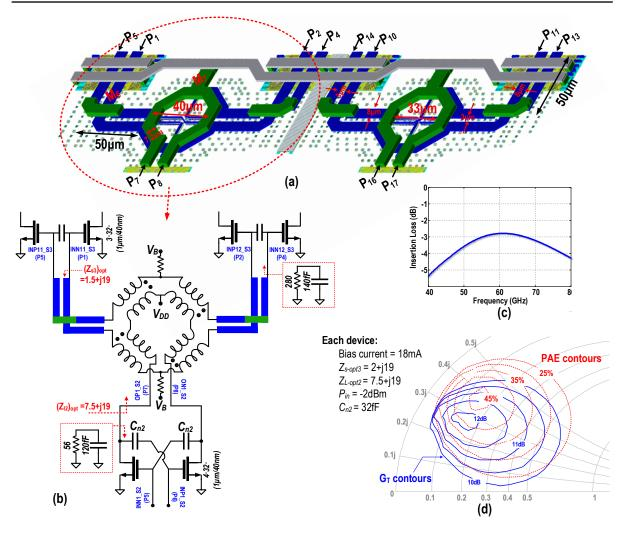
Figure 6.22: (a) Layout of the driver matching network; (b) simplified schematic of the driver amplifier; (c) constant  $G_p$  and PAE contours for  $4.32 \cdot (1 \mu \text{m}/40 \text{nm})$  device; (d) insertion loss of the driver matching network.
