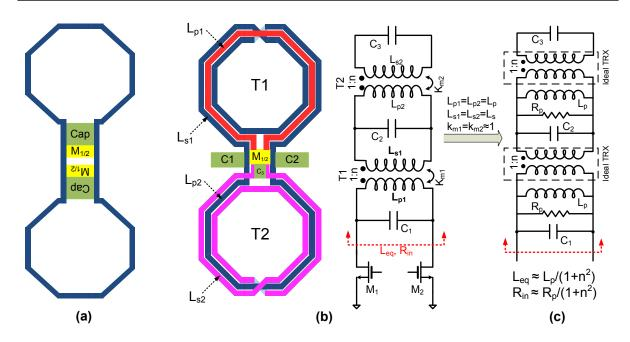
Figure 4.1: Phase noise reduction techniques without sacrificing tank's Q-factor: (a) coupled oscillators, (b) connecting two step-up transformers back-to-back, and (c) its equivalent circuit model.
