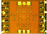
A wideband 60GHz class-E/F<sub>2</sub> PA in 40nm [RFIC2015]
