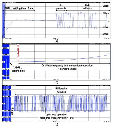
Figure 7.24: (a) ADPLL settling; (b) oscillator frequency drift and (c) demodulated TX frequency for  $425 \,\mu$ sec BLE packet in the open-loop operation.
