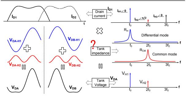
Figure 4.5: Proposed oscillator waveforms in time and frequency domains.
