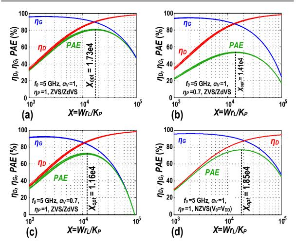
Figure 5.4: Drain, gain and power added effeciency for different flavors of class-E/F PA versus X-factor for technology parameters of  $\overline{R_{on}} = 850 \,\Omega\mu m$ .
