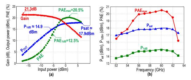
Figure 6.32: (a) Measured gain, output power and power added efficiency versus input power; (b) Measured  $P_{sat}$ ,  $P_{1dB}$  and PAE across frequency.
