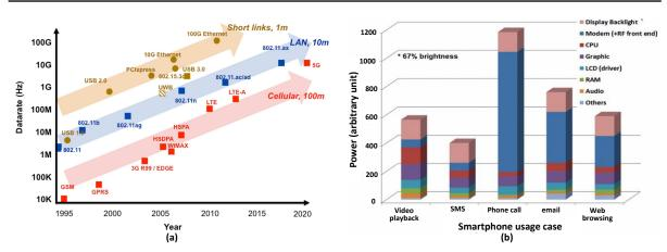
Figure 1.1: (a) evolution of data rates for wireless LAN, cellular, and wireline short links over time [1]; (b) power usage in a smartphone [2].
