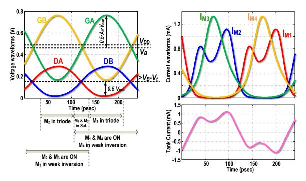
Figure 7.9: Waveforms and various operational regions of  $M_{1-4}$  transistors across the oscillation period.
