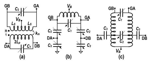
Figure 7.7: Various options of a tank providing voltage gain.
