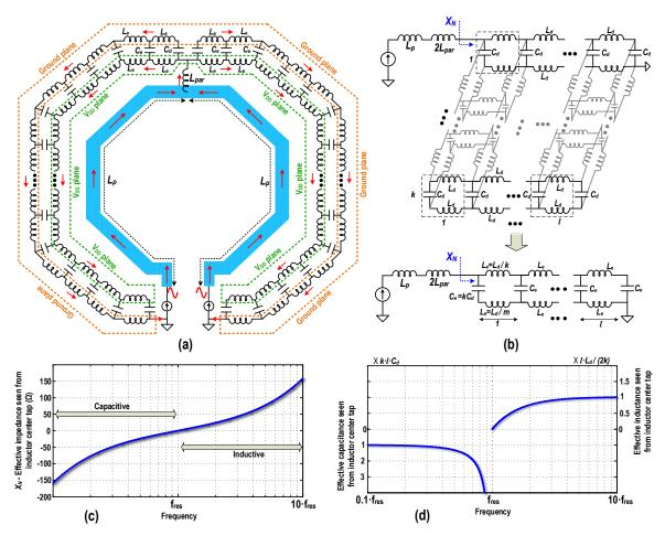
Figure 6.15: (a) Simplified layout and (b) equivalent circuit model of the effective CM inductance seen by PA transistors; (c, d) effective impedance of the bypass network.
