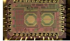
An ultra-low phase noise class-F<sub>2</sub> oscillator in 65nm [RFIC2013, JSSC2015]
