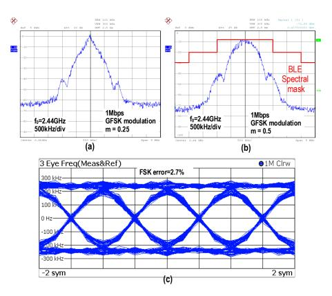
Figure 7.23: Bluetooth GFSK modulation spectrum for modulation index of (a) m=0.25, (b) m=0.5, and (c) burst-mode modulation accuracy.
