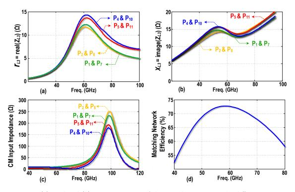
Figure 6.19: (a) Real and (b) imaginary parts of the impedance seen at the different input ports of the output matching network; (c) CM input impedance; (d) passive efficiency of the output matching network.
