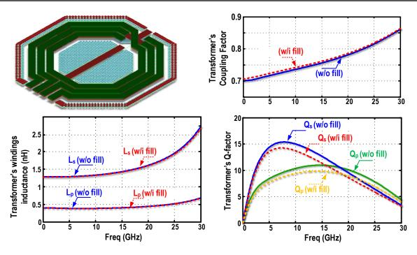
Figure 3.5: Effects of dummy metal fills on the 28 nm CMOS class-F transformer.
