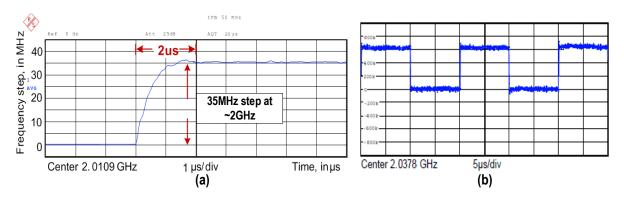
Figure 3.11: (a) Measured demodulated signal during FSK modulation and (b) Measured lock-in time for a frequency step of 35 MHz.
