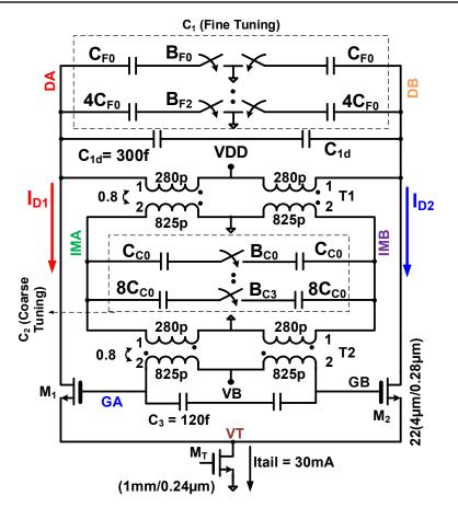
Figure 4.10: Proposed transformer-based class-F<sub>2</sub> oscillator schematic.
