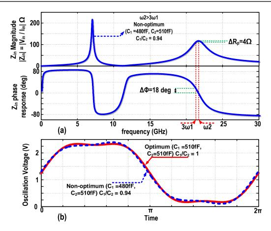
Figure 2.16: Sensitivity of class-F oscillator to the position of the second resonant frequency: tank's input impedance magnitude and phase (top), oscillation waveform (bottom).
