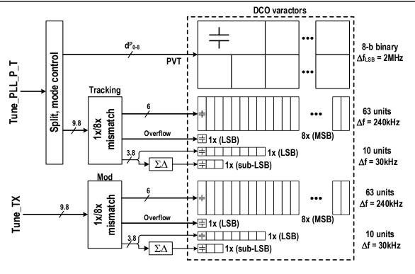
Figure 3.7: The input interface of the proposed DCO.
