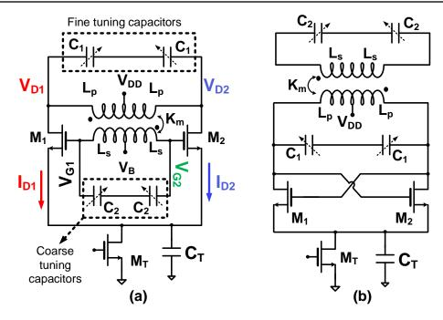
Figure 2.10: Two options of the transformer-based class-F oscillator: (a) transformer-coupled; and (b) cross-coupled. The first option was chosen as more advantageous in this work.
