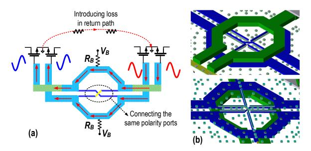
Figure 6.28: (a) Damping the undesired combination of CM and DM oscillation; (b) layout of the proposed transformer-based splitter.
