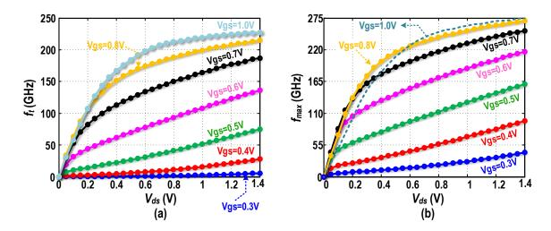
Figure 6.7: Simulated (a)  $f_t$  and (b)  $f_{max}$  of a 96·1 $\mu$ m/40nm with extrinsic interconnect parasitics versus  $V_{ds}$  for different  $V_{qs}$ .
