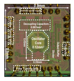
Figure 2.17: Die photograph of class-F oscillator.
