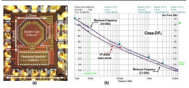
Figure 4.24: (a) Die micrograph of class- $D/F_2$  oscillator; (b) its measured phase noise.
