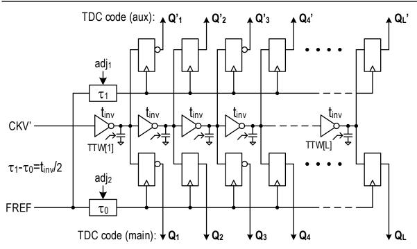
Figure 3.2: Schematic of the parallel TDC with stabilized inverter delay.
