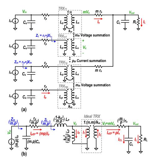
Figure 7.15: (a) Transformer-based matching network with m-way voltage and p-way current summation; and (b) its equivalent circuit model.
