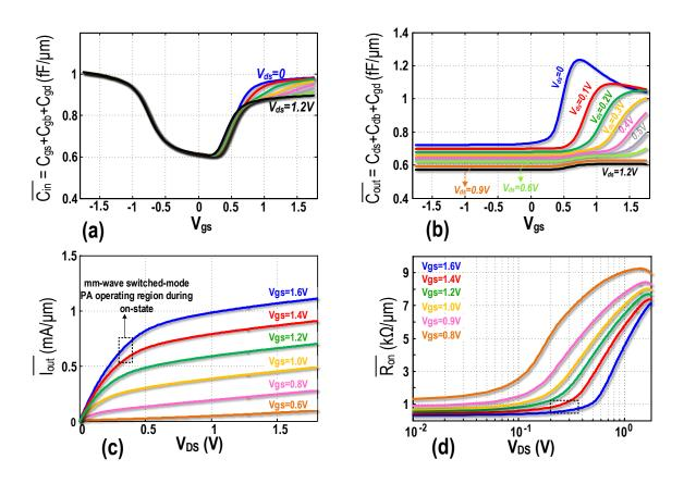
Figure 5.3: Technology dependent parameters in 40 nm CMOS technology, (a)  $\overline{C_{in}}$  and (b)  $\overline{C_{out}}$  versus  $V_{gs}$  for different  $V_{ds}$ , (c)  $\overline{I_{out}}$  and  $\overline{R_{on}}$  versus  $V_{ds}$  for different  $V_{gs}$ .
