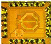
A 0.5mW Switching Current Source Oscillator in 40nm [RFIC2015]
