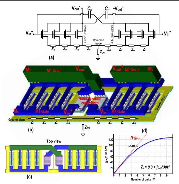
Figure 6.6: (a) Schematic and (b, c) layout of the neutralized differential amplifier; (d) the overall transconductance of the large device versus the number of unit transistors.
