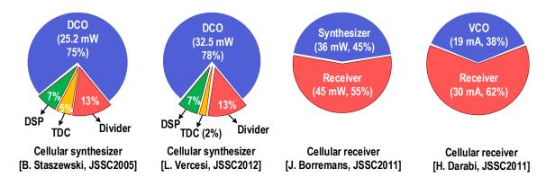
Figure 1.2: Contribution of RF oscillator to the power consumption of cellular frequency synthesizers and receivers.
