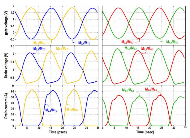
Figure 6.20: Different waveforms of output transistors at 58 GHz.
