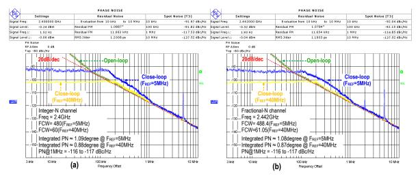
Figure 7.21: Measured transmitter phase noise in open-loop and different close-loop configurations for (a) integer-N and (b) fractional-N channels.
