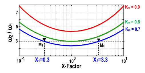
Figure 2.7: Ratio of the tank resonant frequencies versus X-factor for different  $k_m$ .
