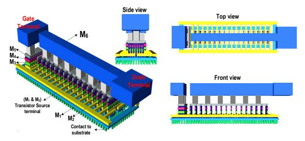
Figure 6.4: Optimal layout of  $32 \cdot 1 \mu m/40 nm$  transistor.
