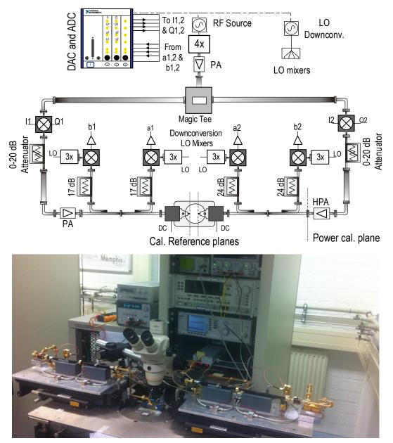
Figure 6.31: Mixed-signal active load-pull setup for large-signal measurements [144].
