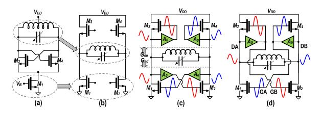
Figure 7.6: Evolution towards the switching current-source oscillator.
