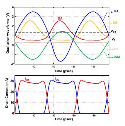
Figure 4.11: Simulated oscillation waveforms of the class- $F_2$  oscillator at  $V_{DD}=1.2$  V and  $I_{DC}=29$  mA: (top) oscillation voltage of different circuit nodes, (bottom) core transistors drain current.
