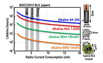
Figure 7.1: BLE system lifetime versus radio current consumption for various battery types.
