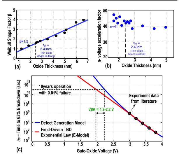
Figure 5.8: (a) Weibull slope versus gate oxide thickness extracted from [14], (b) voltage acceleration versus gate oxide thickness extracted from measurement results in [98], (c)  $\eta_B$  versus gate-oxide voltage. The data points (solid circles) are extracted from literature [110].
