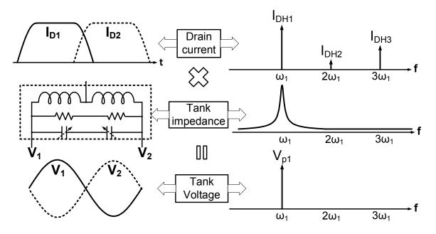
Figure 2.3: Traditional oscillator waveforms in time and frequency domains.
