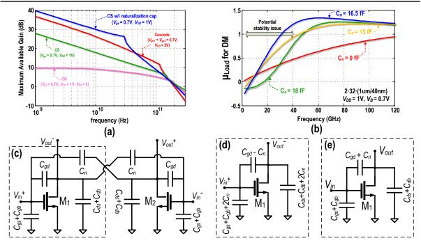
Figure 6.9: (a) Simulated maximum available gain for different amplifier structures; (b) Edwards-Sinsky stability factor for differential amplifier with various  $C_n$ ; (c) neutralized differential amplifier with its parasitic capacitances; Equivalent model for parasitic capacitances of a neutralized transistor in (d) DM and (e) CM excitation.
