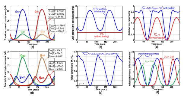
Figure 7.12: Circuit-to-phase noise conversion across the oscillation period in the switching current-source oscillator. Simulated (a) Channel conductance of  $M_{1-4}$ ; (b) Conductance due to resistive losses; (c) Noise factor due to losses; (d) Transconductance of  $M_{1-4}$ ; (e) Effective noise factor due to transconductance gain; (f) Effective noise factors due to different oscillator's components.
