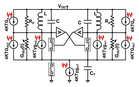
Figure 2.14: RF CMOS oscillator noise sources.
