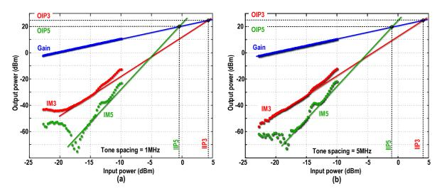
Figure 6.33: Measured two-tone intermodulation for the PA with tone frequency spacing of (a) 1 MHz and (b) 5 MHz.
