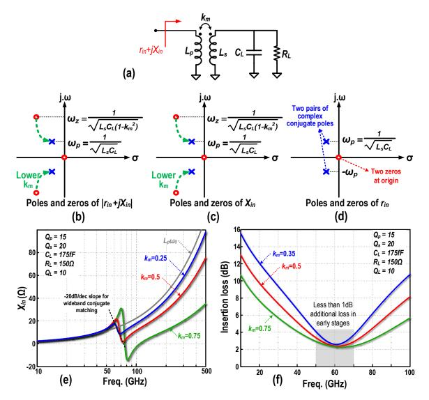
Figure 6.21: (a) Transformer for inter-stage matching; poles and zeros of (b)  $|Z_{in}|$ , (c)  $X_{in}$  and (d)  $r_{in}$ ; (e)  $X_{in}$  and (f) transformer power transfer efficiency versus frequency for different  $k_m$ .
