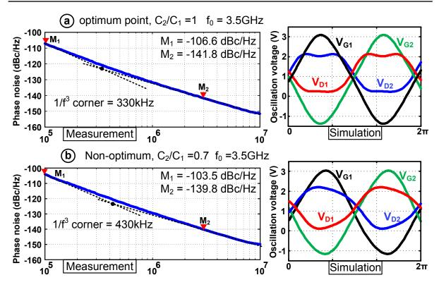
Figure 2.20: Measured phase noise at 3.5 GHz and simulated oscillation waveforms: (a) optimum case; (b) exaggerated non-optimum case.
