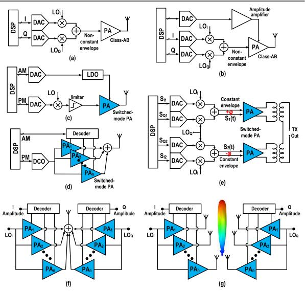
Figure 6.2: Different transmitter architectures: (a) traditional analog-intensive I/Q; (b) Envelope tracking; (c) analog-intensive polar; (d) digitally-intensive polar; (e) outphasing; (f) digitally intensive I/Q structure with on-chip and (g) spatial combining.
