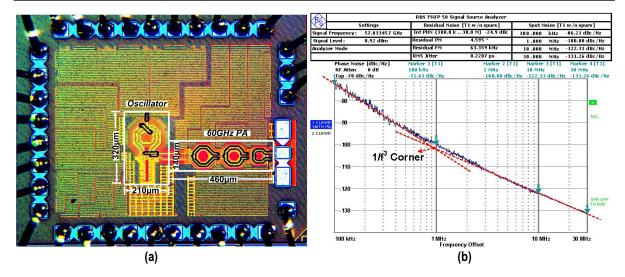
Figure 2.23: (a) Chip micrograph; (b) Measured phase noise at 57.8 GHz.
