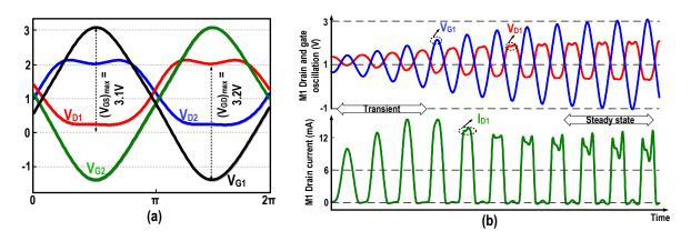
Figure 2.12: (a) Oscillation voltage waveforms and (b) transient response of the class-F oscillator.
