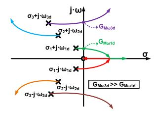
Figure 4.12: Root-locus plot of the class- $F_2$  oscillator.
