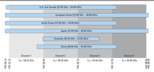
Figure 6.1: 60 GHz band channel plan and frequency allocations by region [112].
