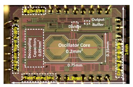
Figure 4.15: Die photograph of the class- $F_2$  oscillator.
