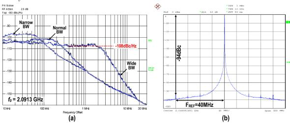
Figure 3.9: Measured ADPLL (a) phase noise and (b) spectrum (a); with 40 MHz FREF. The spectrum, taken with wide loop bandwidth of 1.5 MHz, is virtually spur-free.
