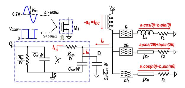
Figure 5.1: Generalized schematic of class-E/F power amplifier including NMOS device circuit model as a switch.
