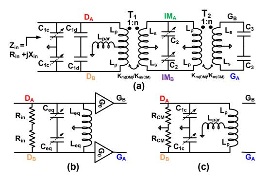
Figure 4.8: Proposed transformer-based resonator: (a) schematic, (b) its simplified equivalent differential-mode circuit ( $k_{m(DM)} \approx 1$ ), (c) simplified tank schematic for common-mode input signals ( $k_{m(CM)} \approx 0$ ).
