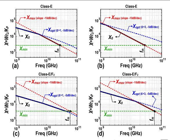
Figure 5.5:  $X_{opt}$ ,  $X_{min}$ ,  $X_{max}$  and  $X_0$  of class-E and class-E/F<sub>2</sub> PA over frequency. ( $\overline{R_{on}} = 850 \,\Omega\mu m$ ,  $\overline{C_{in}} = 1 \, fF/\mu m$ ,  $\overline{C_{out}} = 0.65 \, fF/\mu m$ ,  $\overline{I_{out}} = 0.6 \, mA/\mu m$ )
