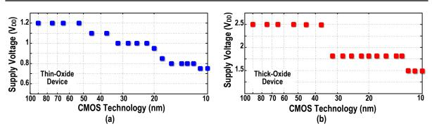
Figure 1.3: Nominal supply voltage versus CMOS technology node for (a) thin-oxide and (b) thick-oxide device.
