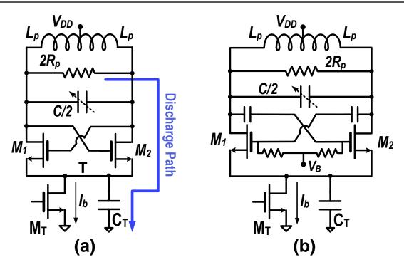
Figure 2.1: Oscillator schematic: (a) traditional class-B; (b) class-C.
