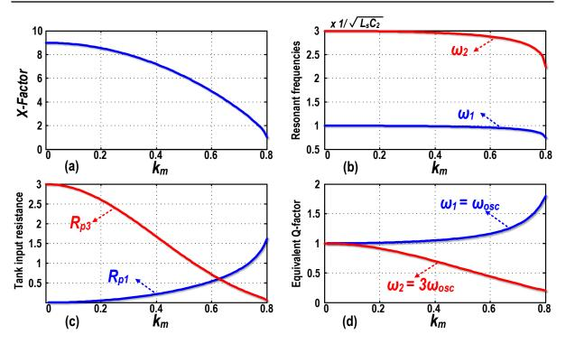
Figure 2.22: Dependency of (a) X-factor; (b) tank's first and second resonant frequencies; (c)  $R_{p1}$  and  $R_{p3}$ ; (d) tank's equivalent Q-factor on  $k_m$  (while  $\omega_2/\omega_1 = 3$ ).
