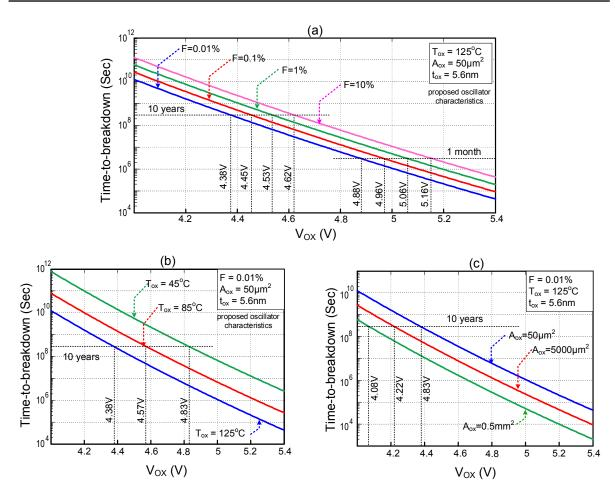
Figure 4.20: Estimated time-to-breakdown (based on the measured parameters of Fig. 4.19(a)) of thick-oxide transistors in 65 nm CMOS versus maximum gate-oxide stress voltage for different (a) cumulative failure rates, (b) temperatures, (c) gate-oxide areas.
