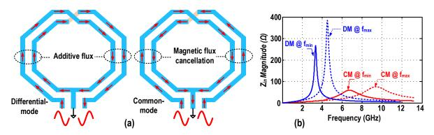
Figure 4.22: Proposed  $F_2$  inductor in DM and CM excitation (top),  $F_2$  tank and its input impedance (bottom).
