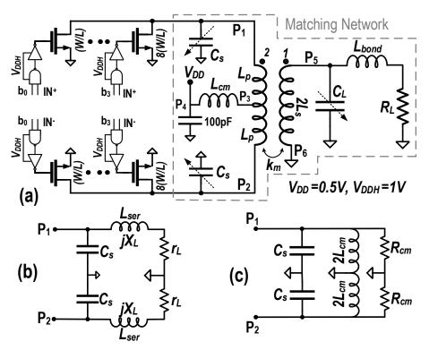
Figure 7.14: (a) Schematic of the proposed class-E/F<sub>2</sub> PA. Equivalent circuit PA's matching network for (b) differential, and (c) common-mode excitations.
