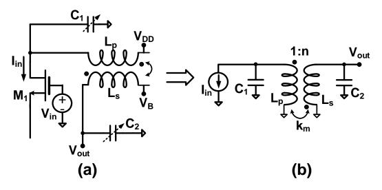
Figure 2.13: Open-loop circuit for unloaded Q-factor calculation (a); its equivalent circuit (b).
