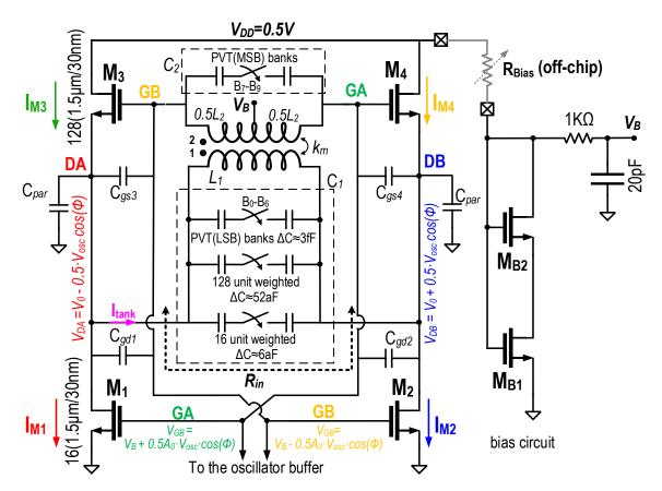
Figure 7.8: Schematic of the proposed switching current-source oscillator.
