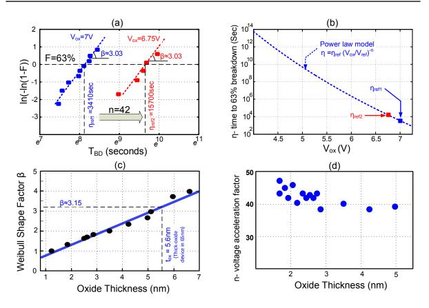
Figure 4.19: (a) Measured cumulative failure rate F versus breakdown time  $T_{BD}$  for 14 samples of a thick-oxide transistor  $(176\mu m/0.28\mu m)$  at room temperature, (b) the projected  $\eta$  value versus different gate-oxide stress voltage based on the measured  $\eta_{ref}$ , (c) Weibull slope versus gate oxide thickness extracted from measurement results in [14], (d) voltage acceleration versus gate oxide thickness extracted from measurement results in [98].
