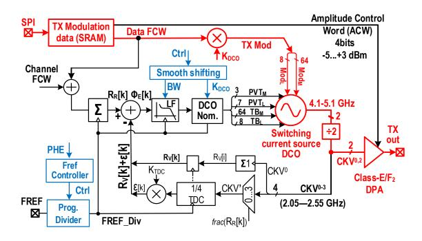
Figure 7.18: Block diagram of the 2.4 GHz ULP Bluetooth Low-Energy transmitter.
