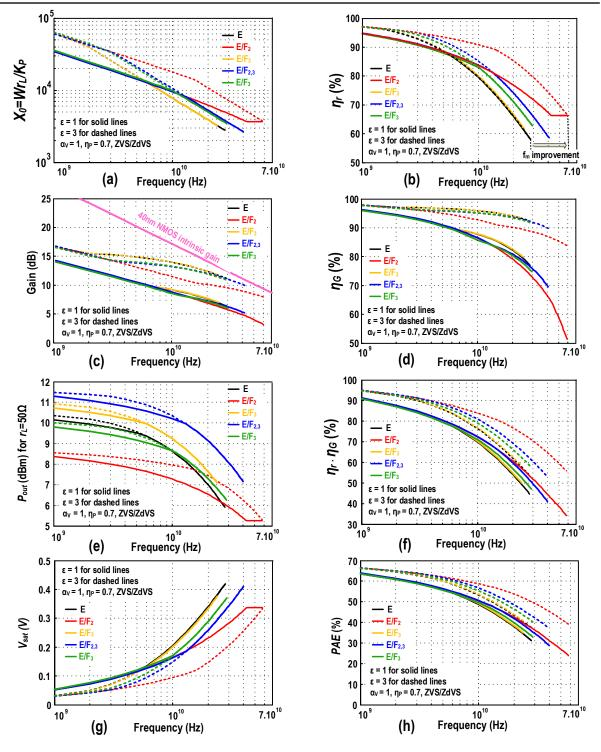
Figure 5.6: Characteristics of different flavors of class-E/F PA versus frequency at the maximum achievable PAE. (40 nm TSMC LP technology:  $\overline{R_{on}} = 850 \,\Omega\mu m$ ,  $\overline{C_{in}} = 1 \, fF/\mu m$ ,  $\overline{C_{out}} = 0.65 \, fF/\mu m$ ,  $\overline{I_{out}} = 0.6 \, mA/\mu m$ )
