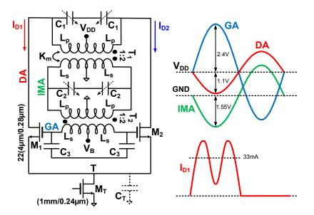
Figure 4.2: Preliminary oscillator schematic and its simulated voltage and estimated current waveforms at  $f_0=8 \text{ GHz}$ ,  $V_{DD}=1.2 \text{ V}$ ,  $I_{DC}=33 \text{ mA}$ ,  $L_{eq}=80 \text{ pH}$  and  $C_{eq}=4.95 \text{ pF}$ .
