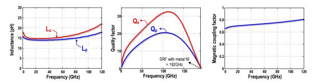
Figure 6.12: Different characteristics of the transformer used in the output matching network.
