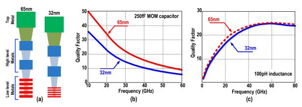
Figure 1.4: (a) Back-end-of-line (BEOL) metallization; quality factor of (b) a 250 fF capacitor, and (c) a 100 pH inductor in 65 nm and 32 nm CMOS technologies [16].
