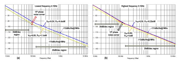
Figure 7.20: Measured phase noise of the proposed oscillator at (a) lowest and (b) highest frequency.
