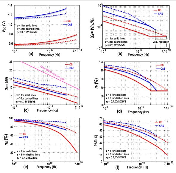
Figure 5.10: Characteristics of single-divice and cascode class-E/F<sub>2</sub> PA versus frequency at the maximum achievable PAE. ( $\overline{R_{on}} = 850 \,\Omega\mu m$ ,  $\overline{C_{in}} = 1 \, fF/\mu m$ ,  $\overline{C_{out}} = 0.65 \, fF/\mu m$ ,  $\overline{I_{out}} = 0.6 \, mA/\mu m$ ,  $V_{BK} = 2 \,\mathrm{V}$ )
