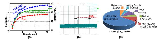
Figure 7.25: (a) PA characteristics; (b) TX harmonic emissions; and (c) TX power breakdown at  $P_{out}=0$  dBm.
