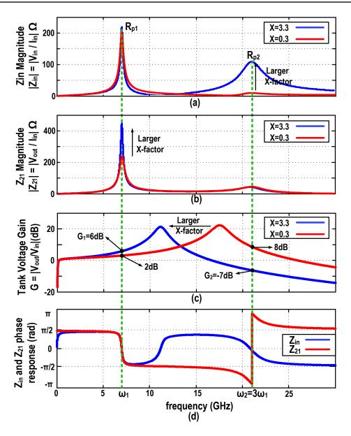
Figure 2.8: The transformer-based tank characteristics: (a) the input impedance,  $Z_{in}$  magnitude; (b) the trans-impedance,  $Z_{21}$  magnitude; (C) transformer's secondary to primary voltage gain; (d) the phase of  $Z_{in}$  and  $Z_{21}$  (Momentum simulation).
