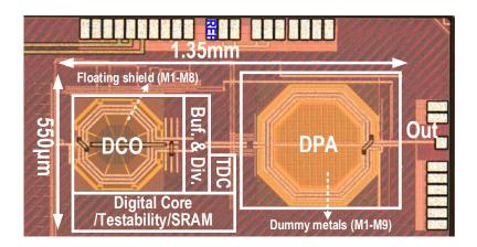
Figure 7.19: Die micrograph of the proposed ULP transmitter.
