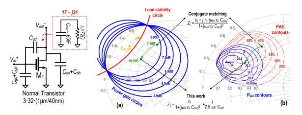
Figure 6.18: (a) Load stability circle and constant power gain circles for  $3\cdot32\cdot(1\mu m/40nm)$  transistor; (b) constant PAE and  $P_{sat}$  circles for the last stage with an ideal series-parallel combiner.
