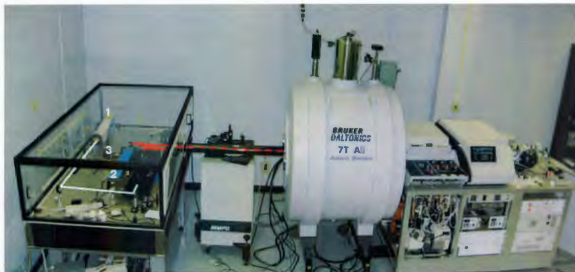
Figure 7.5: FT-ICR MS instrument coupled with an OPO/A laser at Memorial University.
