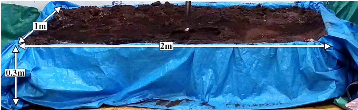
Figure 3-2. Specially-constructed box filled with planting medium.
