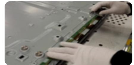
Disassemble the source PCB from the guide
