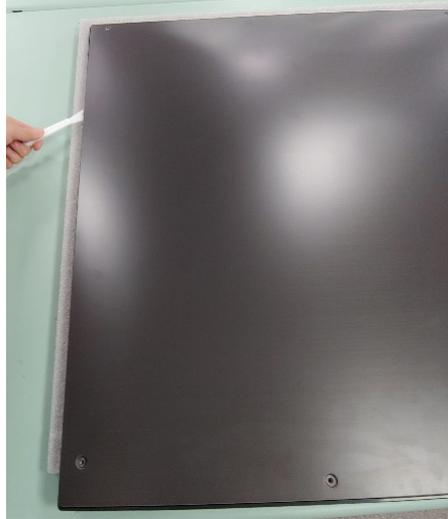
(5) Right Side : Disassemble B/C Using Opener. Put the opener into the gap of guide panel and back cover and move upward.
