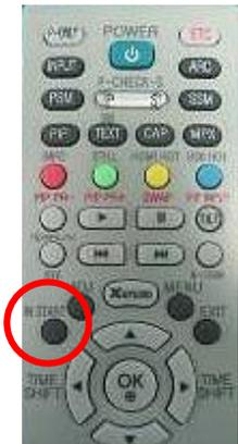
Press the IN-START with the remote control for adjustment
