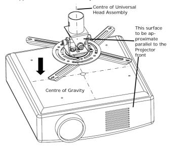
2A.3— Place the Bottom Spacers in between the Extension Brackets and the Projector, and align the mounting holes as shown below.
