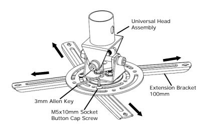
2A.2— Place projector's Flush Mount Assembly over the projector and align the centre of the Flush Mount with the projector's approximate Centre of Gravity.
