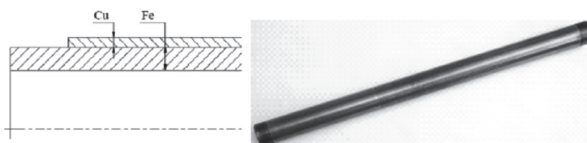
Fig. 10. Tubular rotor of 2DoF induction motor (cross-section and real view)
