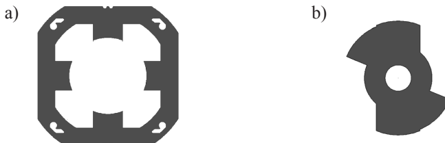
Fig. 1. Geometry of the 4/2 SRM: (a) stator, (b) rotor
