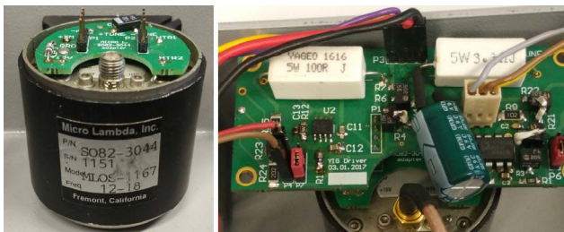
Figure 4. Micro Lambda Inc. Ku band YIG oscillator (a) with a voltage-to-current converter/driver (b)
