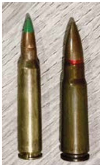
Left: brass casing, Right: lacquer coated steel casing
