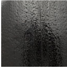
Rows of fine pits, smaller pits between, surface scratched.
