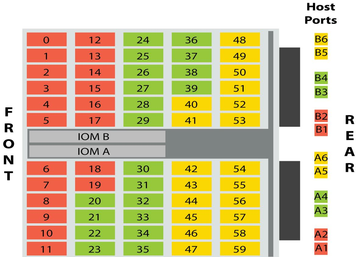
Connect the host servers to the enclosure using SAS cables in the configuration listed in the table below. The left side of the table displays the host number, and the right side displays the appropriate IOM SAS ports on the enclosure for that host.
