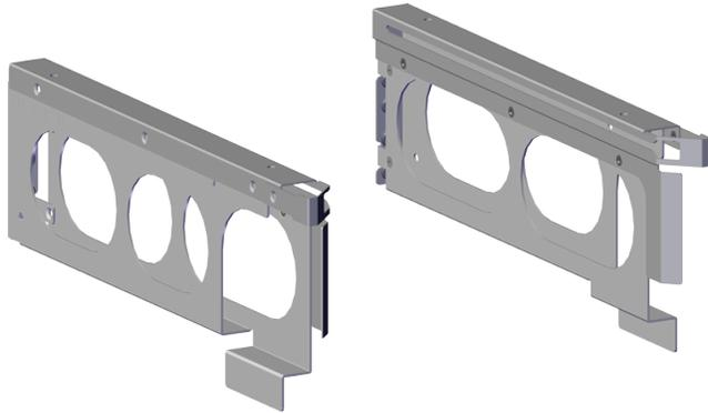
The Rear Cover Alignment Brackets are designed to keep the top cover of the Chassis in the rack while extending the Ultrastar Data60 out of the rack for servicing. The Rear Cover Alignment Brackets attach to the rear vertical rack rails and rest on top of the toolless rail system.
