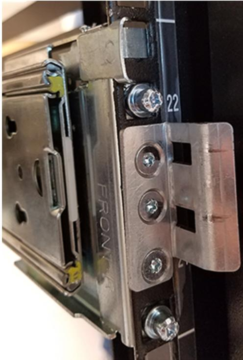
**Step 17:** Uninstall the rack rails from the rack.
