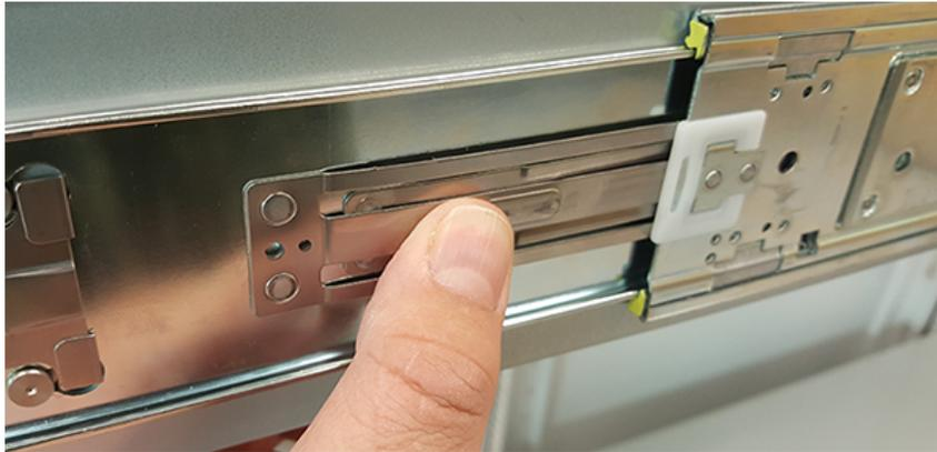
**Step 19:** Push the chassis back into the rack.
