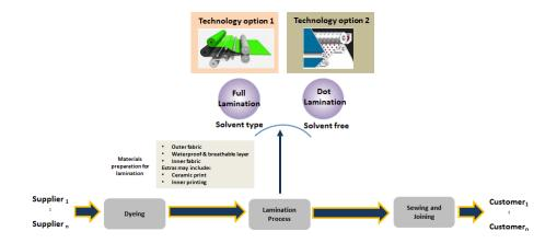
Fig. 3. Full lamination/solvent type and dot lamination/solvent free processes investigated
