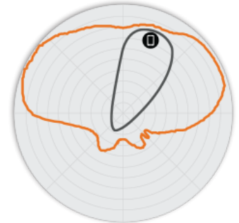
Figure 5. R710 5GHz Elevation Antenna Patterns
