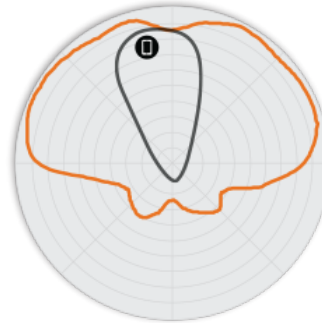
Figure 4. R710 2.4GHz Elevation Antenna Patterns
