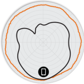
Figure 2. R710 2.4GHz Azimuth Antenna Patterns
