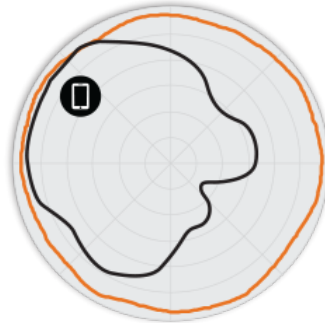
Figure 3. R710 5GHz Azimuth Antenna Patterns
