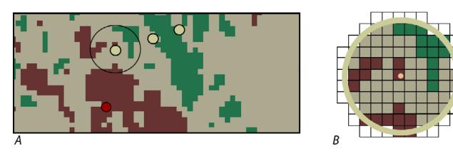
**Figure 4–1.** Detailed view of ground-truth data, showing accuracy-assessment methodology. *A*, Dots illustrate ground-truth observation points, each of which represents 10-second window of substrate observation plotted over seafloor-character grid; circle around dot illustrates area of buffer depicted in *B*. *B*, Pixels of seafloor-character data within 10-m-radius buffer centered on one individual ground-truth video observation.
