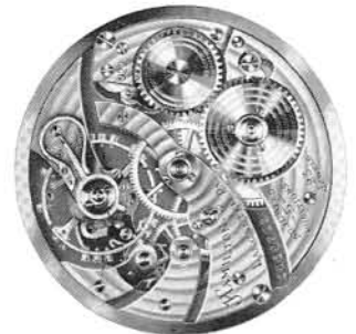
GRADE 922 Open face, bridge movt., 23 jewels, double roller
