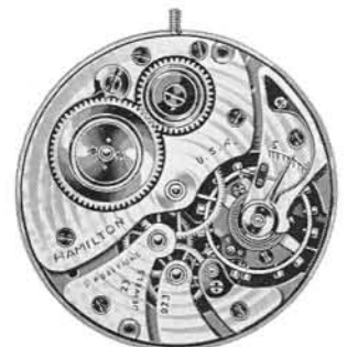
GRADE 923 Open face, bridge movt., 23 jewels, double roller
