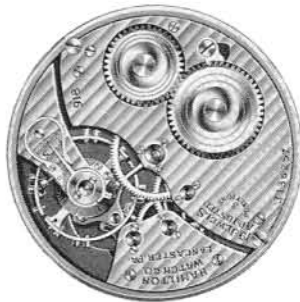
GRADE 918 Open face, \frac{3}{4} plate movt., 19 jewels, double roller
