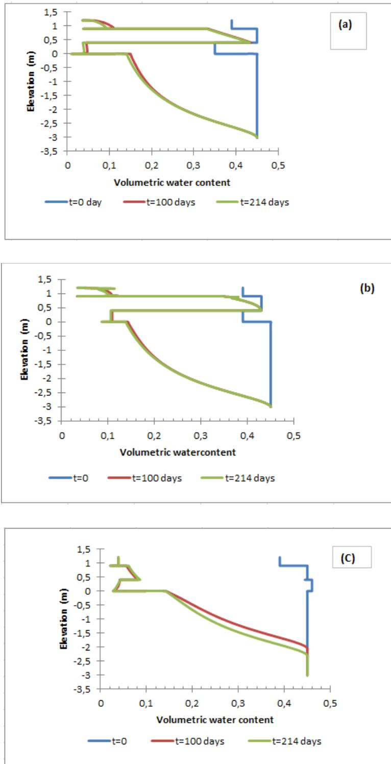
**Figure 4-13** : Volumetric water content evolution with the -3 m water table of (a) column 1 with waste rock (0-20 mm) in the bottom CBL; (b) column 2 with waste rock (0-50 mm) in the bottom CBL; and (c) column with sand S-2 in the bottom CBL.
