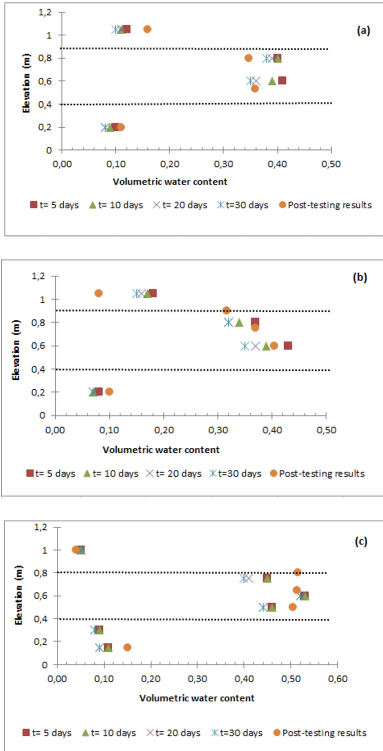
**Figure 4-7 :** Comparison between volumetric water content measurements obtained at the post-testing stage and those measured with EC-5 and GS-3 probes during a typical 30 days cycle in the tested layered systems of (a) column 1; (b) column 2; and (c) column 3.
