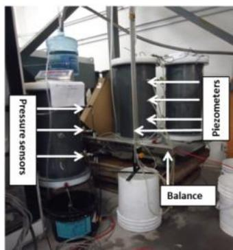
**Figure 4-1** : Column used for permeability and drainage test.
