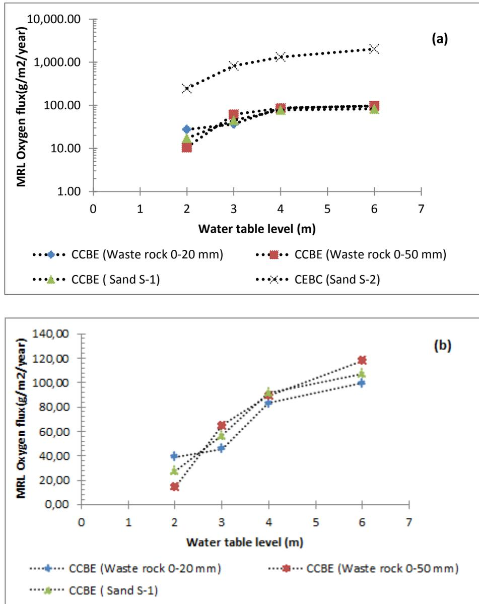
**Figure 4-14 :** Effect of water table position on cumulative oxygen flux at the bottom of the moisture retaining layer (MRL) of the tested CEBCs for (a) natural climatic conditions; (b) extreme climatic conditions.
