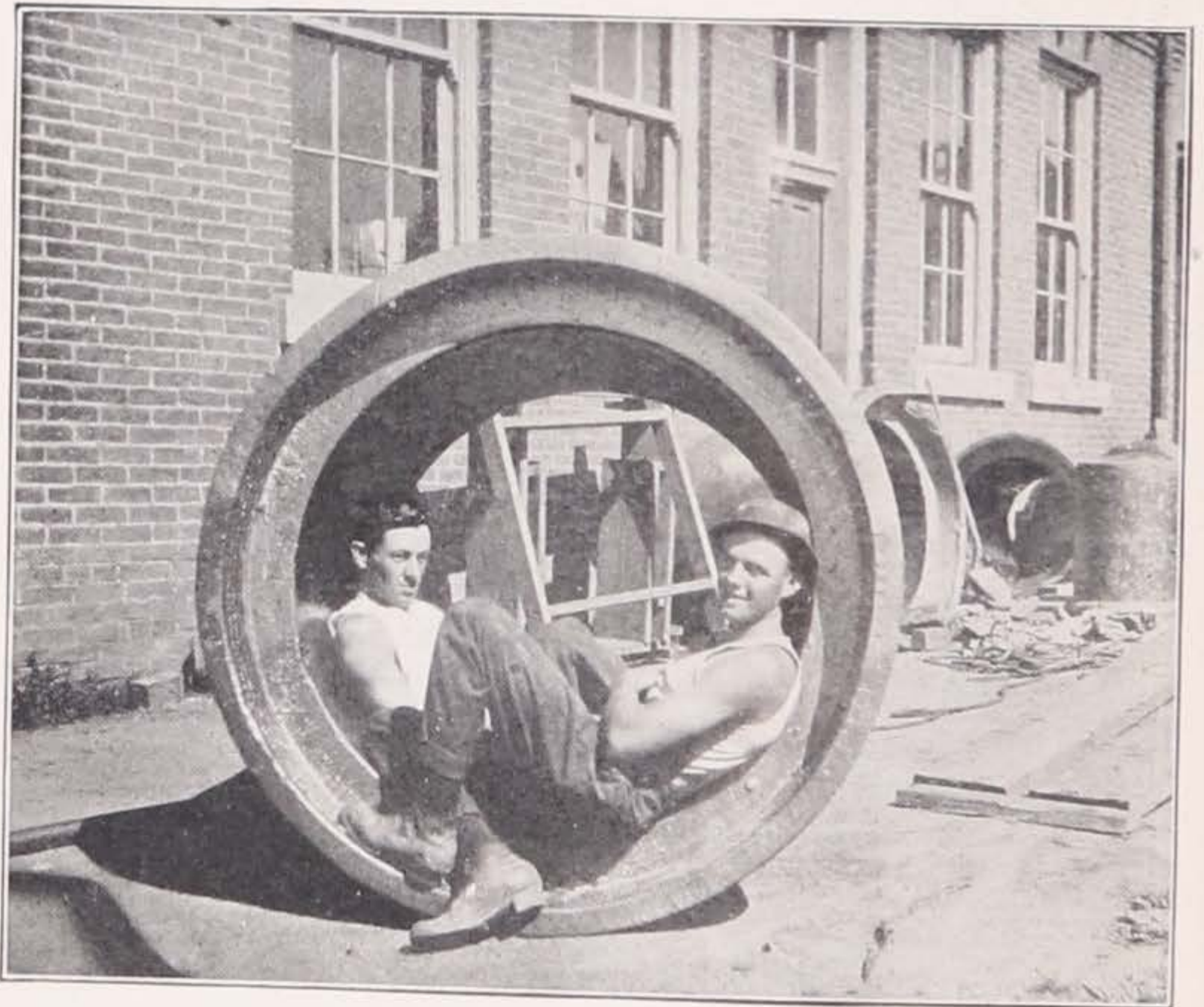
Fig. 25. Forty-two Inch Vitrified Clay Sewer Pipe, about to be Placed in the Testing Machine.
