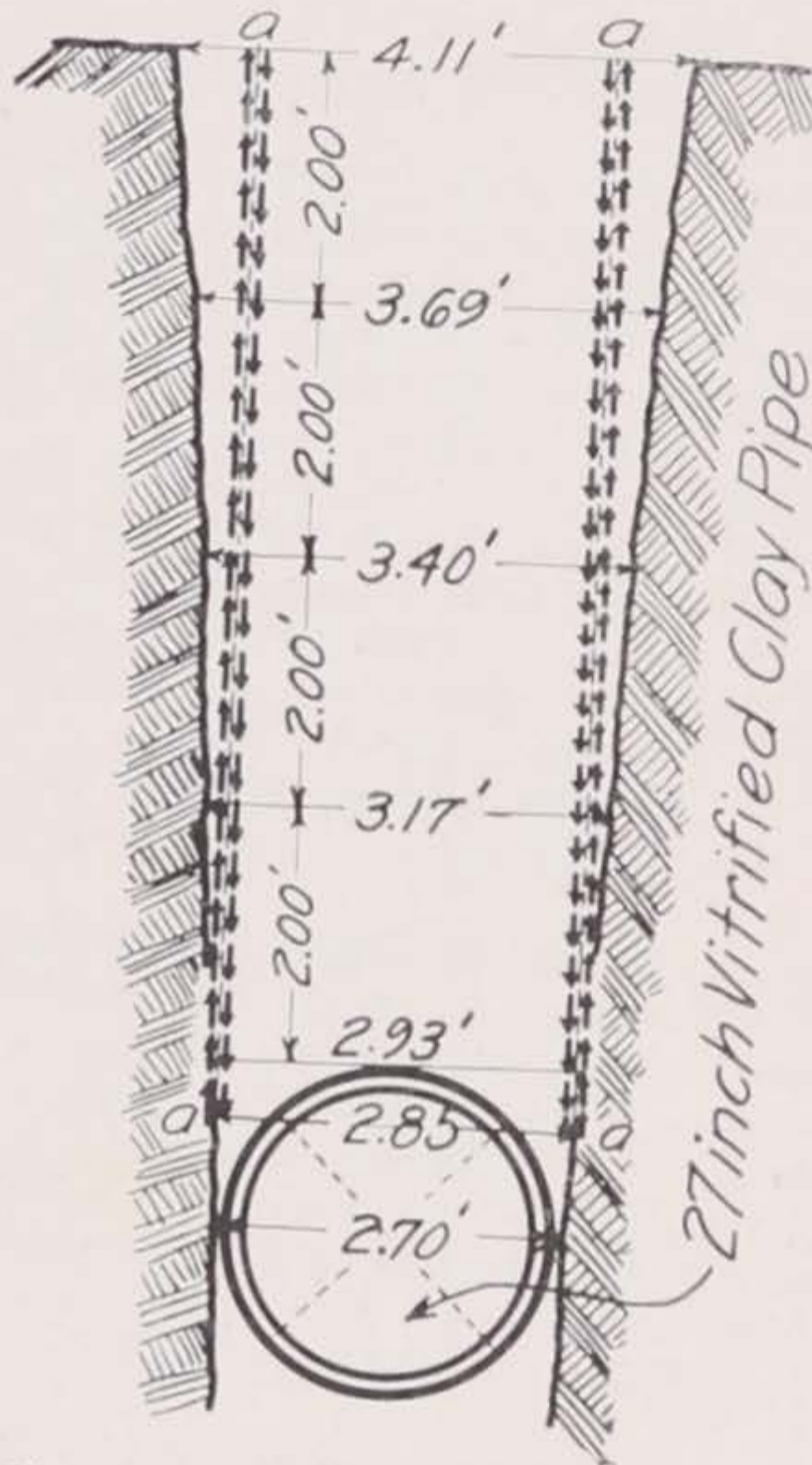
Fig. 16. Scale Drawing of Ditch Used in Experiment No. 8, Table No. 12, page 74, Illustrating Theory of Loads on Pipes in Ditches Wider at the Top than at the Bottom.
